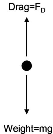
Figure 2: Force acting on the sphere
