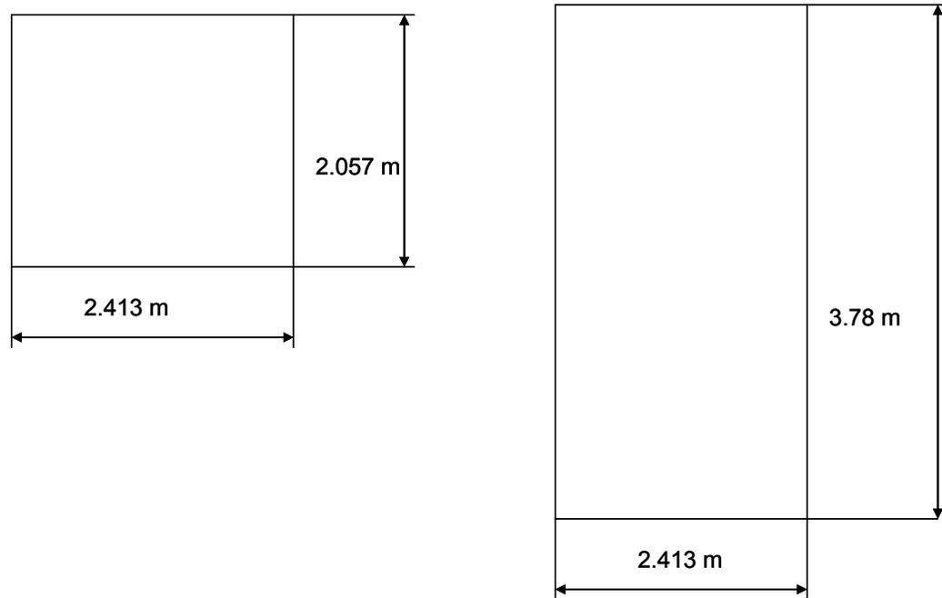
Figure 3 Approximate dimension of the irradiator pool
