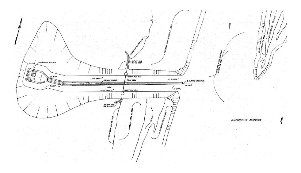
FIGURE 9.4-3 Intake Plant Design Channel from Reservoir to Pumping Station Located in Embayment
