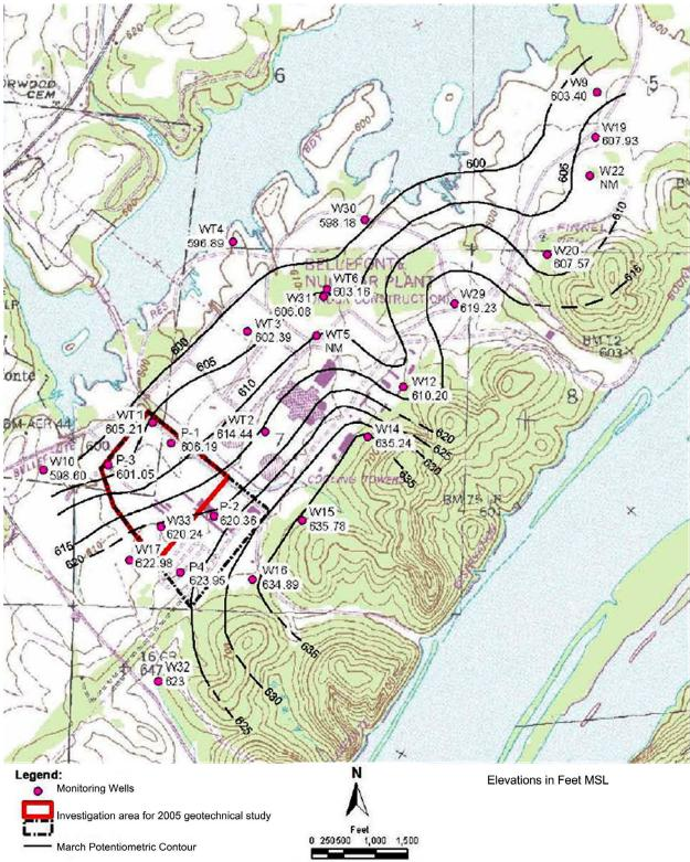
Note: The March 2005 reading from Well W29 is considered an anomalous reading, and the water level and interpretation of the groundwater elevations in the vicinity of Well W29 depicted in this figure are not considered in current groundwater evaluations.
