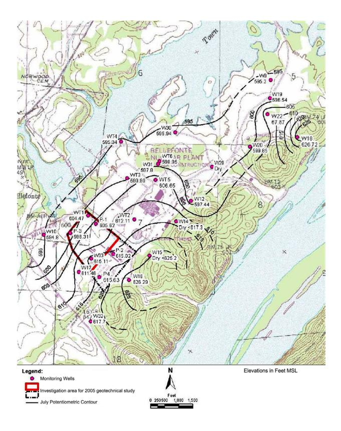
FIGURE 2.3-23 (Sheet 3 of 4) July 2005 Potentiometric Surface Map
