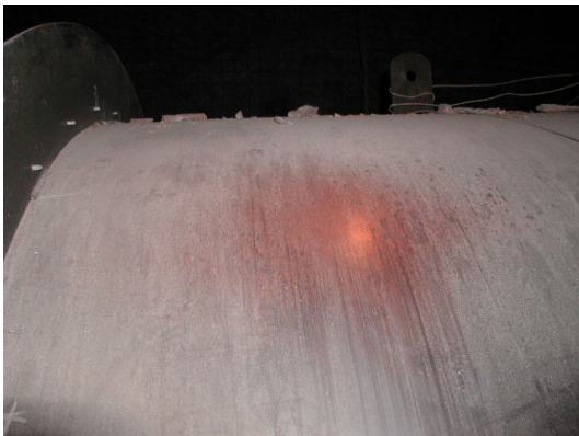
These photos are indications of staining from liquid that dripped onto the surface of a canister heater from the roof of the heated drift.
