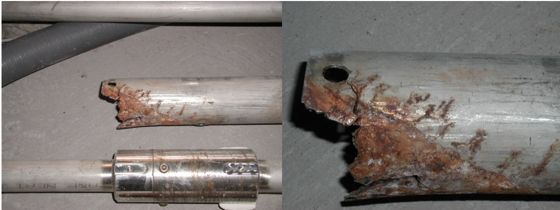
These photos were taken by Kevin Smart on April 18, 2006. They are indicators of the corrosive effect of waters from the rock mass that encounter borehole materials.
