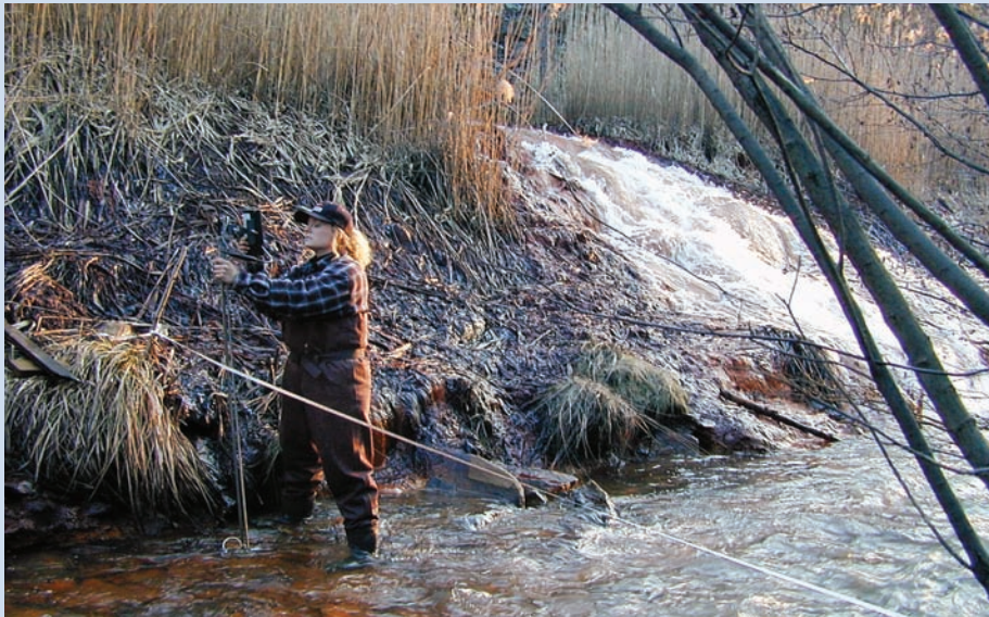
Suzanne Ward, a USGS hydrologic technician, measures the flow rate in Mahanoy Creek, a stream in the Swatara watershed affected by abandoned mine drainage.
