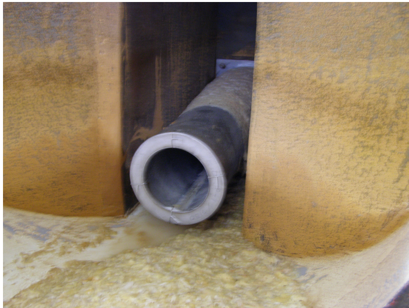
Figure 2. Post-test review of the top-hat strainer showing essentially bare strainer surface on the end opposite the suction side and a settled fiber pile on the pipe bottom upstream of the strainer.
