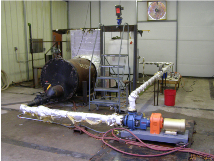
Figure 1. Test loop for 30-day integrated chemical effects head loss test.
