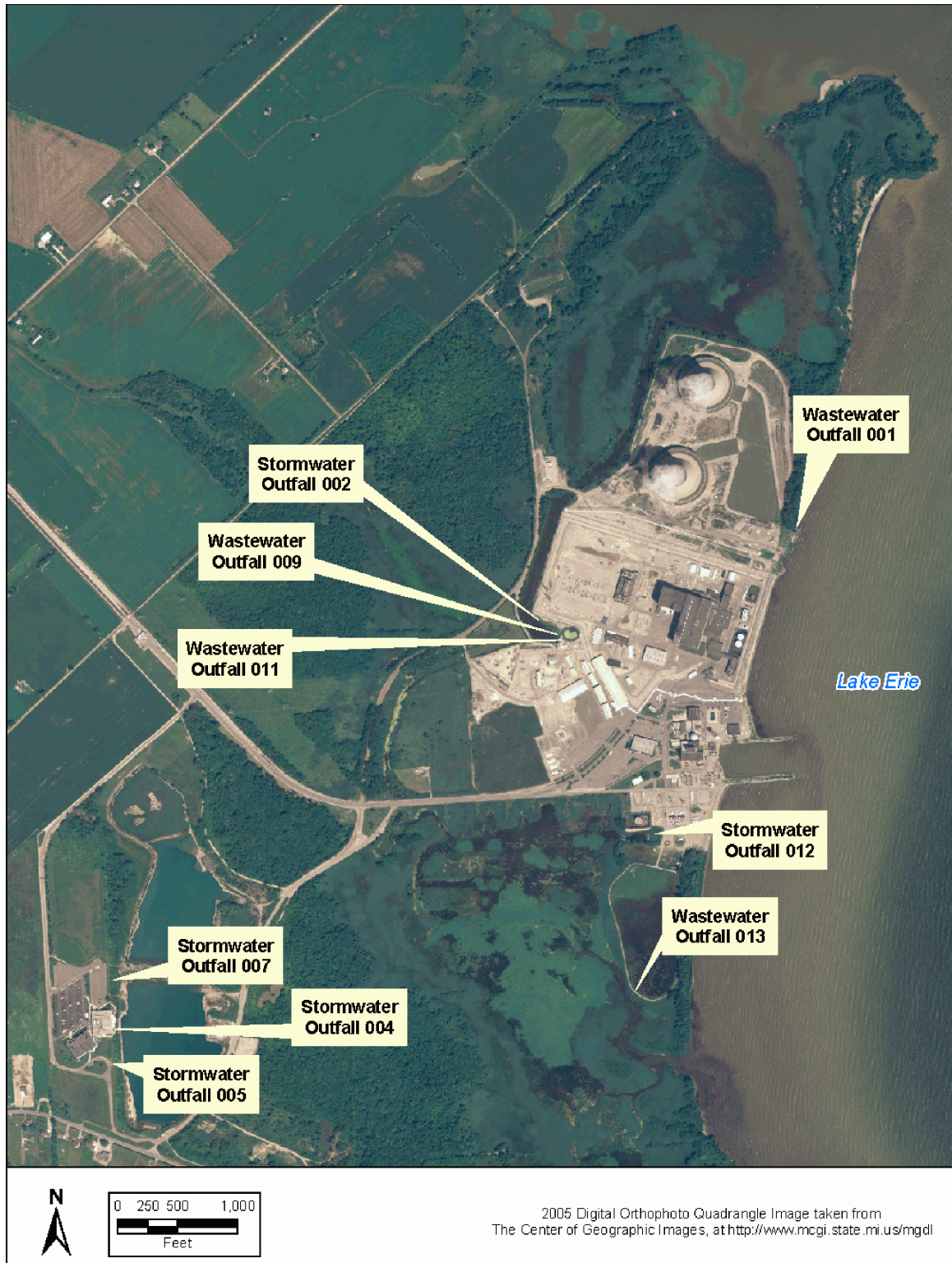
Figure 2.3-47 Permitted Outfalls Located at the Fermi Site
