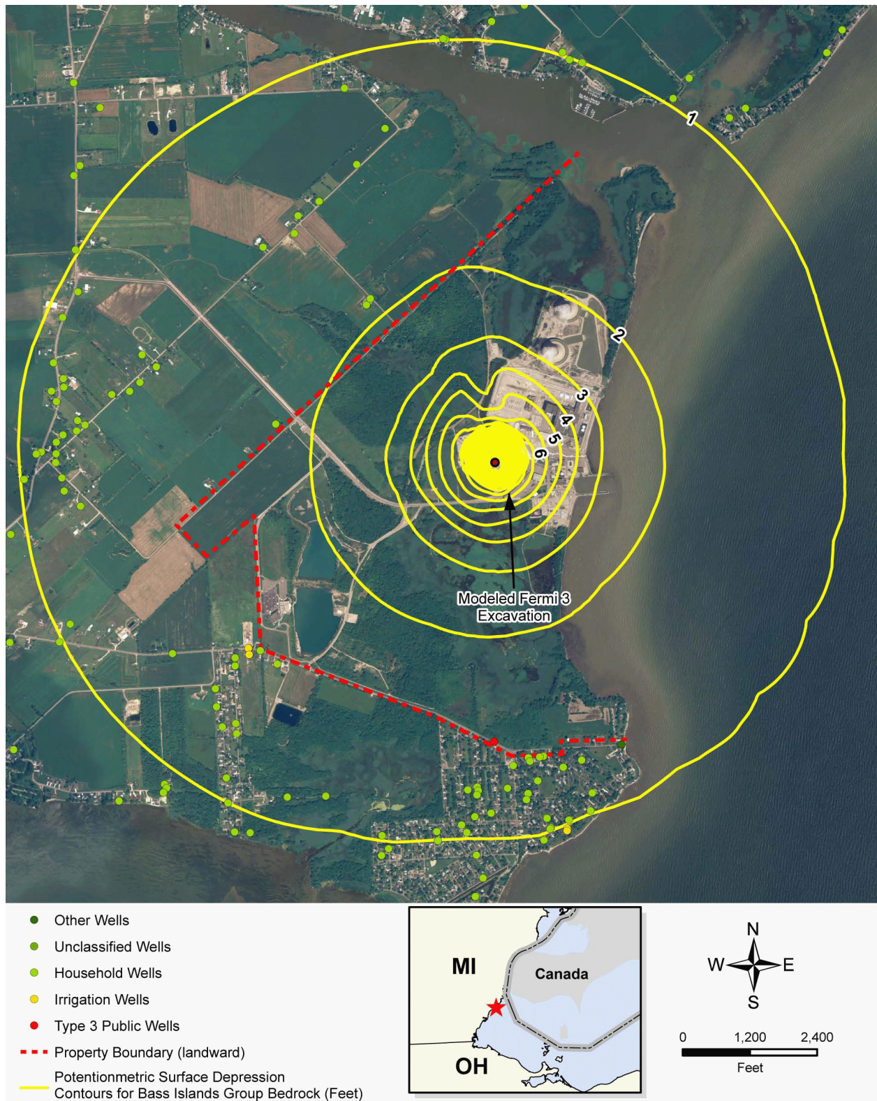
Figure 2.4-256 Dewatering Bass Islands Group: Drawdown Contours – Grout Curtain/Freeze Wall Combination with a Grouted Base
