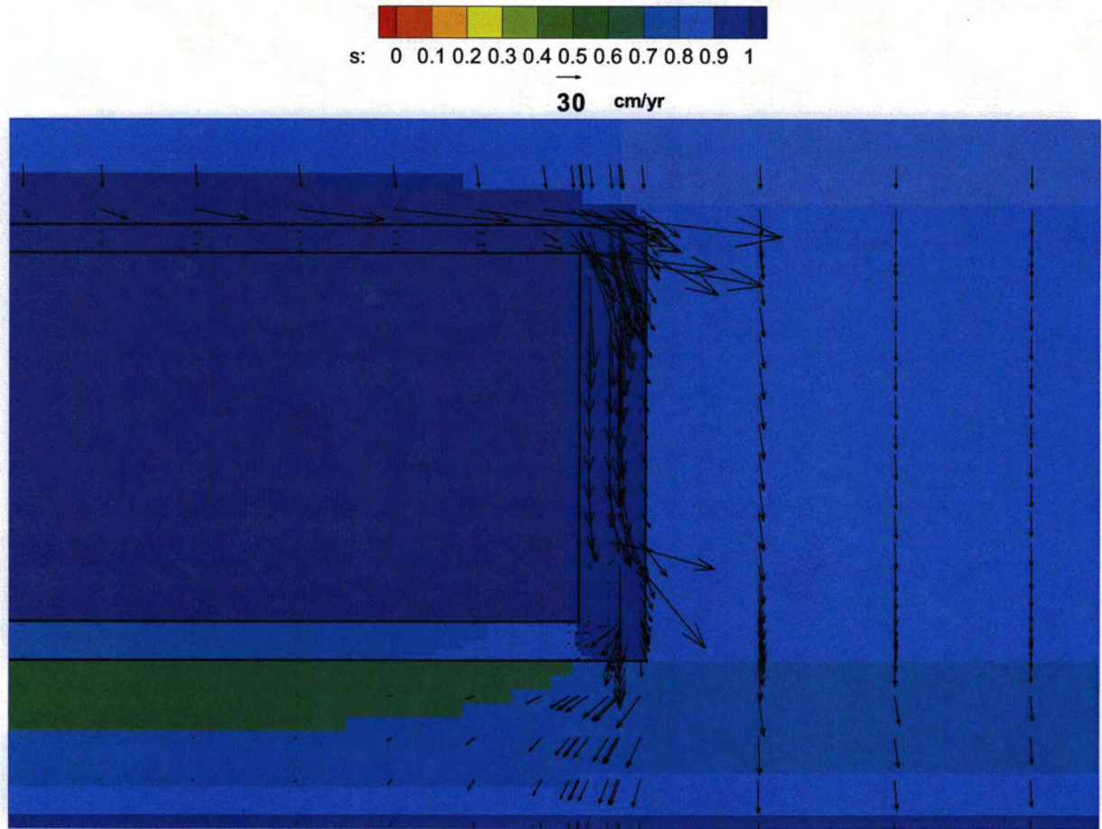
Figure 4.4-23: Type I Tank Flow Field – Immediately Prior to Liner Failure
