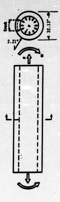
$\frac{Normal Loads}{F_{x} = 1392 \text{ kips}}$  $M_{b} = 10711 \text{ in-kips}$
