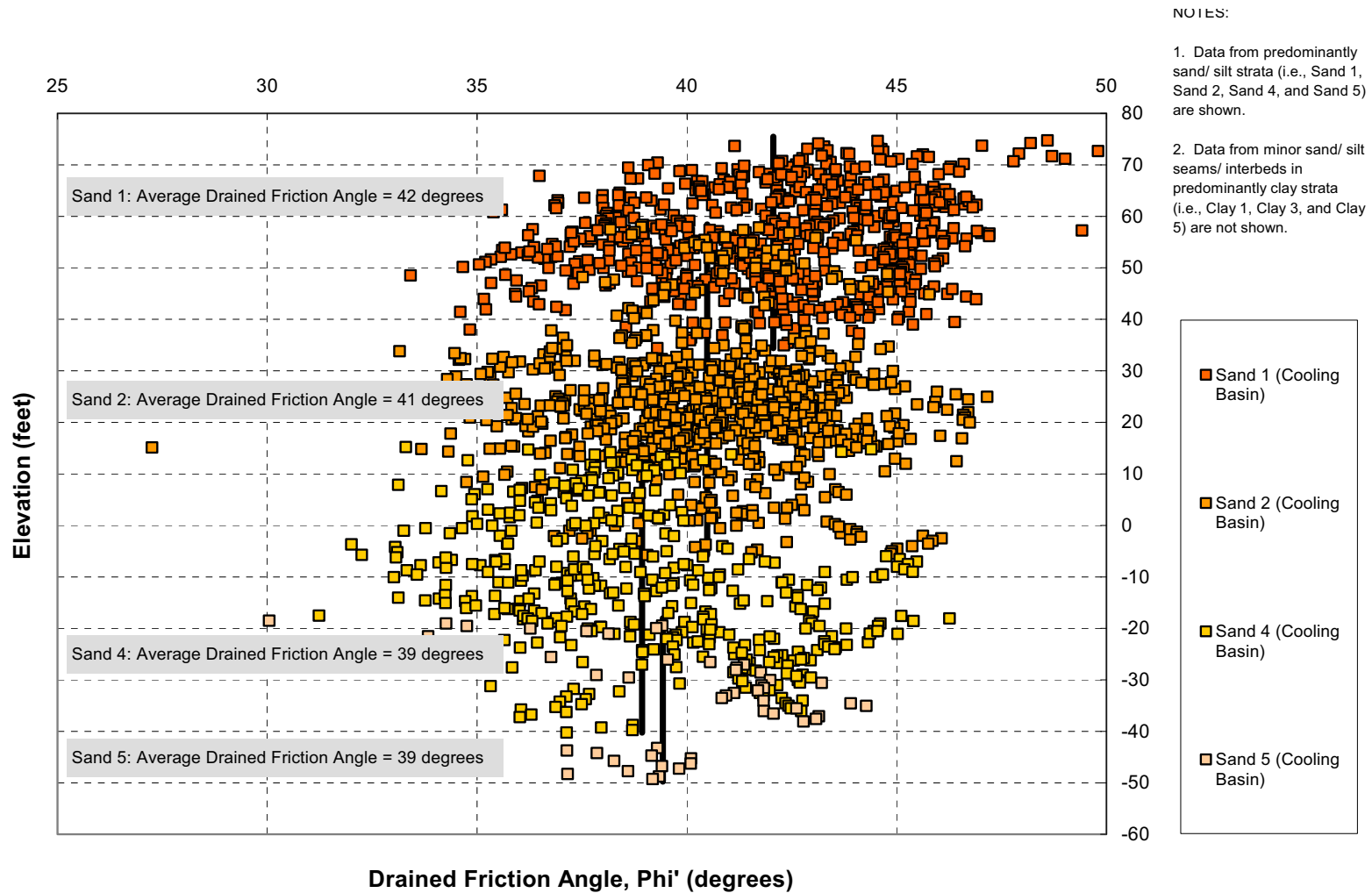
Figure 2.5.4-265 Drained Friction Angles (Phi') of Cohesionless Soil Strata from CPT Data (Cooling Basin/GBRA Storage Water Reservoir)
