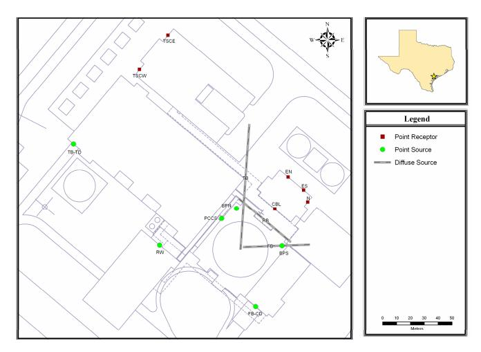
Figure 2.3.4-203 Potential Radiological Sources and Receptors for the ESBWR
