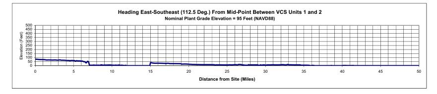
Figure 2.3.2-214 Terrain Elevation Profiles within 50 miles of the VCS Site (Sheet 2 of 6)
