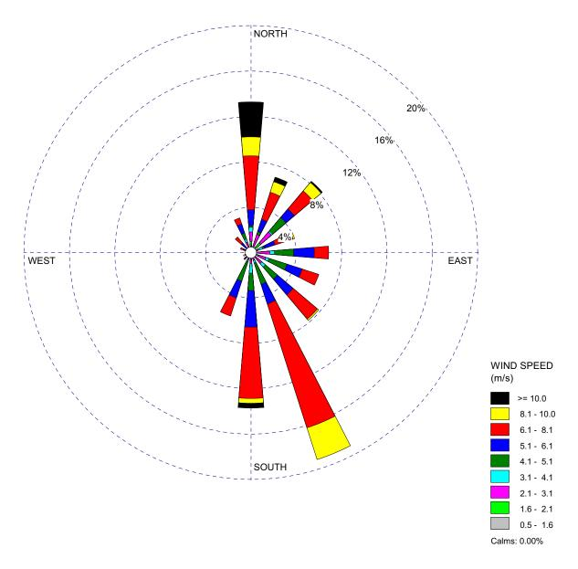
Figure 2.3.2-212 60-Meter Level Wind Rose — November (Sheet 11 of 12) VCS Pre-Application Monitoring Program (July 1, 2007–June 30, 2008)
