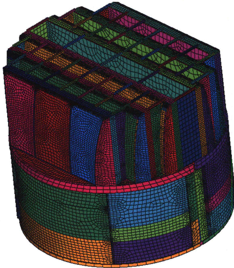
Figure 5a. Mesh overview. The colors emphasize element type.
