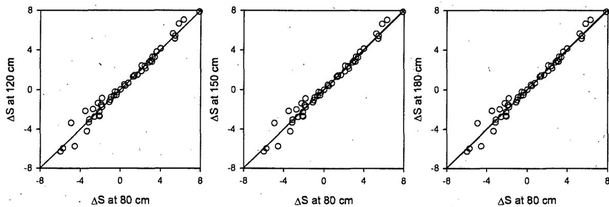
Figure 3-3. Relationships between changes of soil water storage in different soil layers for location BL1.
