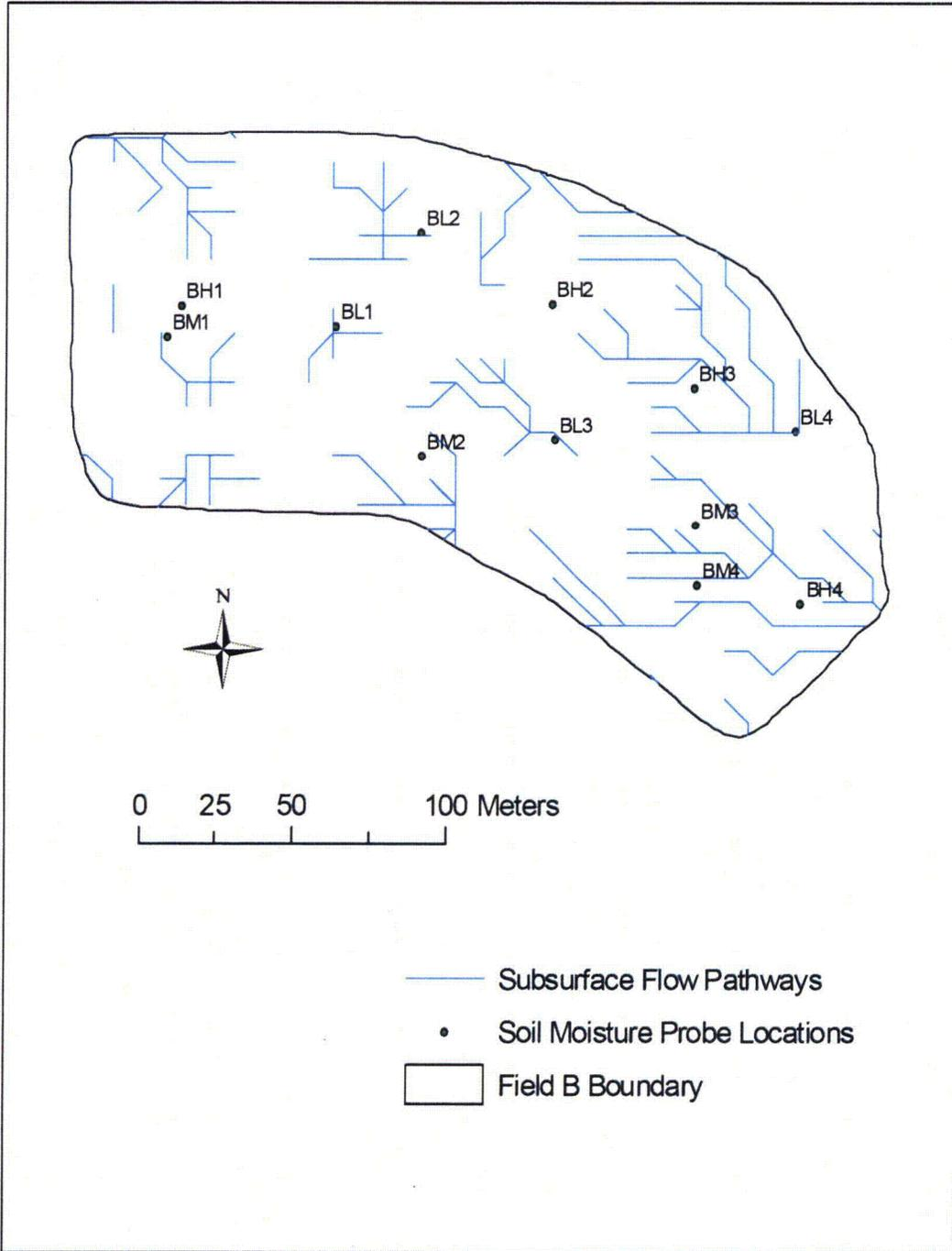
Figure 2-2. Subsurface flow pathways and locations of soil moisture multi-sensor capacitance probes (MCP) in field B.
