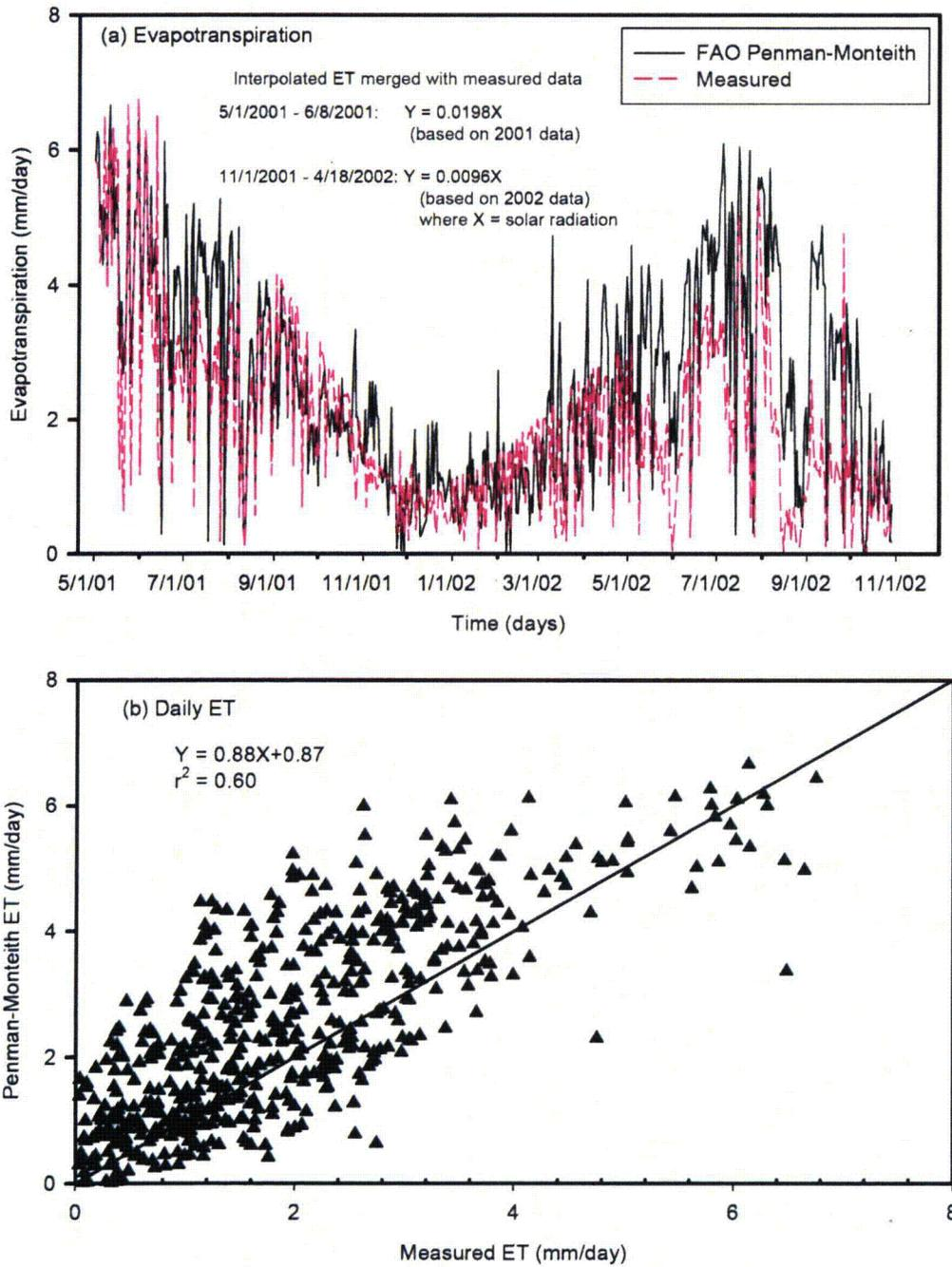
Figure 2-5. Comparison of evapotranspiration calculated using the FAO Penman-Monteith method and measured evapotranspiration using energy budget methods. Evapotranspiration was extrapolated (using solar radiation) for days that did not have measured data (May 1 - June 8, 2001 and January 1 - April 18, 2002).
