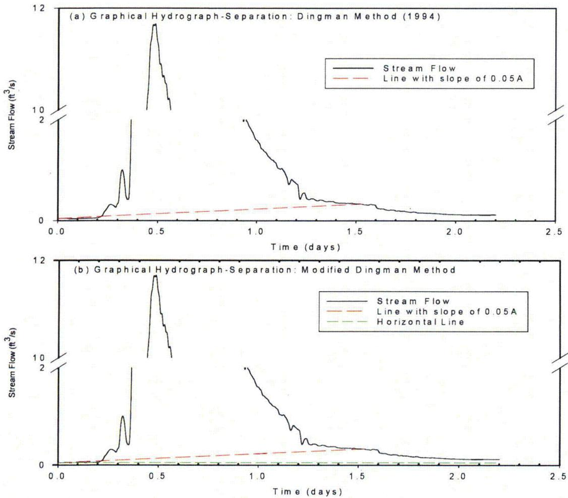
Figure C-1. Graphical stream flow hydrograph separation techniques
