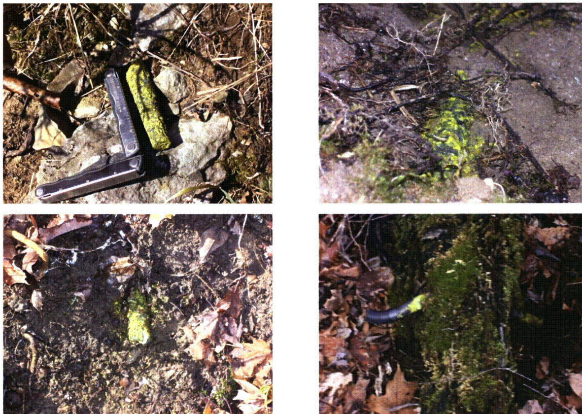
Figure 5-1. DU Penetrators Observed During April 2008 Gamma Walkover Survey
