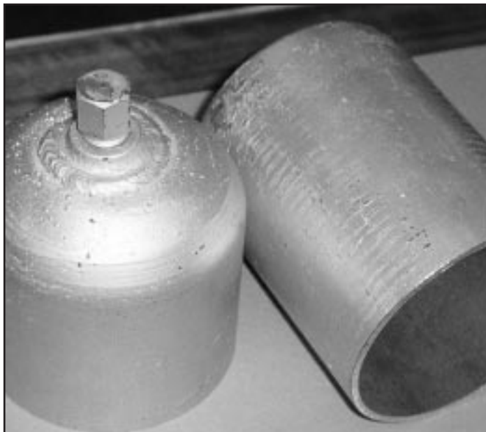
◀ A typical flask is shaped like a cylinder, 5 inches in diameter by 12-15 inches high.
