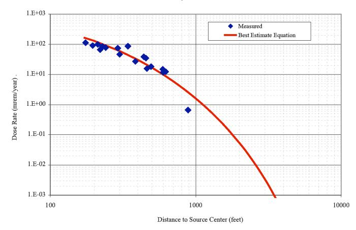
Figure 12.3-5—{Resin Area and ISFSI Historical TLD Readings}
