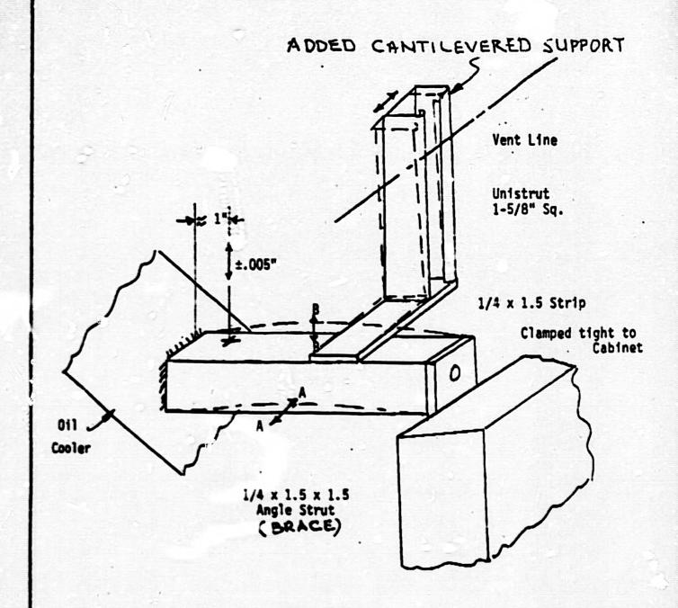
Motions "AA" and "BB" are Torsional Mode in Cooler-Cabinet Strut
