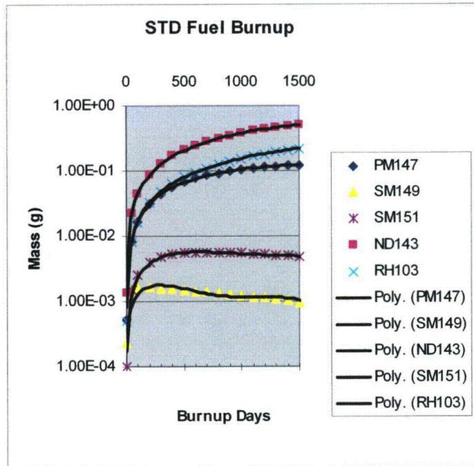
Figure 14 Masses for Typical Heavy Metals and Fission Products – Core 34A
