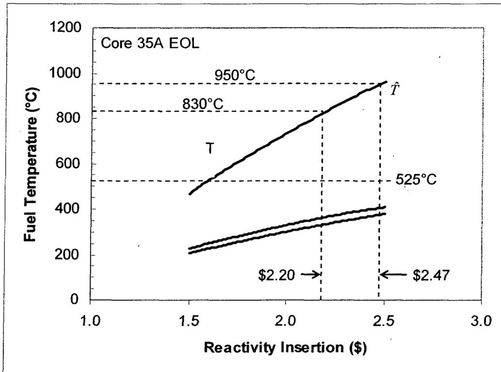
Figure 35 Pulse Performance at 1000 MWD Burnup – WSU Mixed LEU Core 35A
