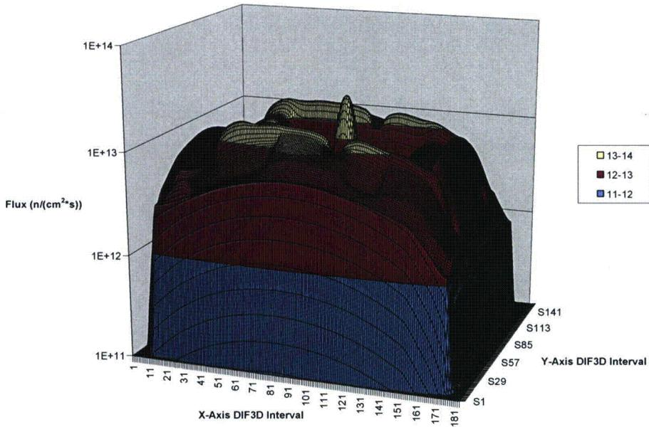
Figure 37 Thermal Neutron Flux ( $E < 0.42$  eV) at fuel axial centerline, BOL, WSU Mixed LEU Core 35A
