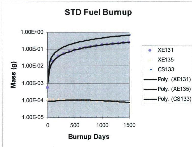
Figure 15 Masses for Typical Heavy Metals and Fission Products – Core 34A
