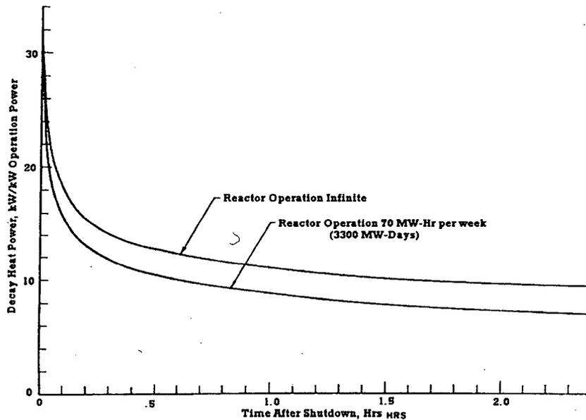
Figure 44: Decay Heat Power Generation Following Loss of Coolant for Infinite Reactor Operation and Periodic Reactor Operation
