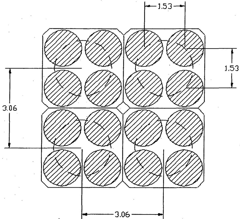
Figure 5 Nominal Fuel Element and Cluster Spacing in the WSU Core (dimensions are inches)
