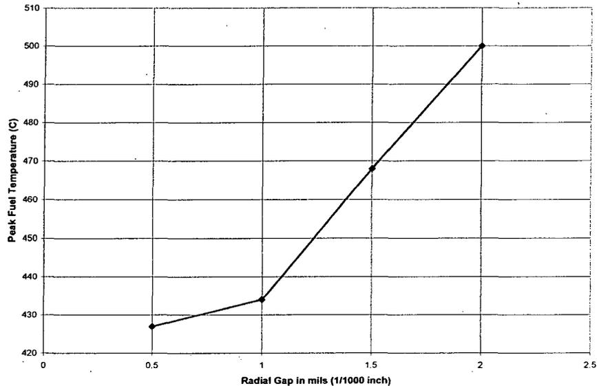
Figure 36 Peak Fuel Temperature as a function of Manufactured Radial Gap
