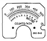
202-643 for Model 16 with any detector 0-500 cpm, 0-2.5 kV OL (overload)
