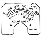
202-558 for Model 4 with any detector 0-500 cpm, 0-2.5kV OR (overrange)
