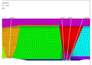
McGuire RPV Outlet Nozzle - Residual Model (With Buffer Layer)
