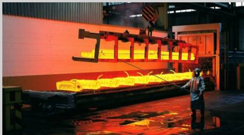
Bars undergoing heat treatment at the Altena plant
