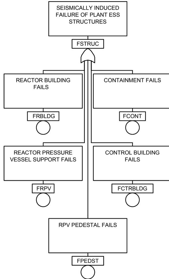
**Figure 15-4. Structural Seismic Fault Tree (Full Power)**
