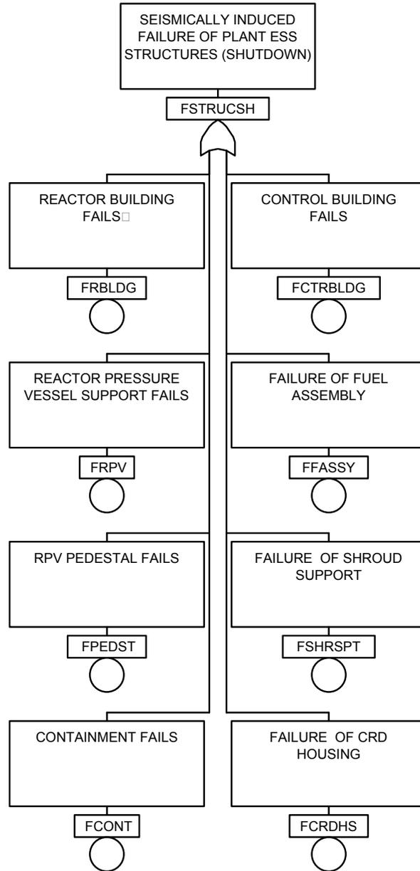
Figure 15-16. Structural Seismic Fault Tree (Shutdown Conditions)
