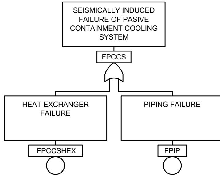
**Figure 15-13. PCCS Seismic Fault Tree**
