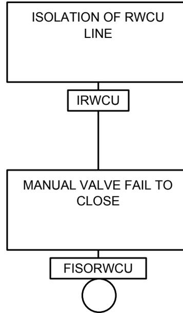
**Figure 15-20. BOC In RWCU Line Fault Tree**
