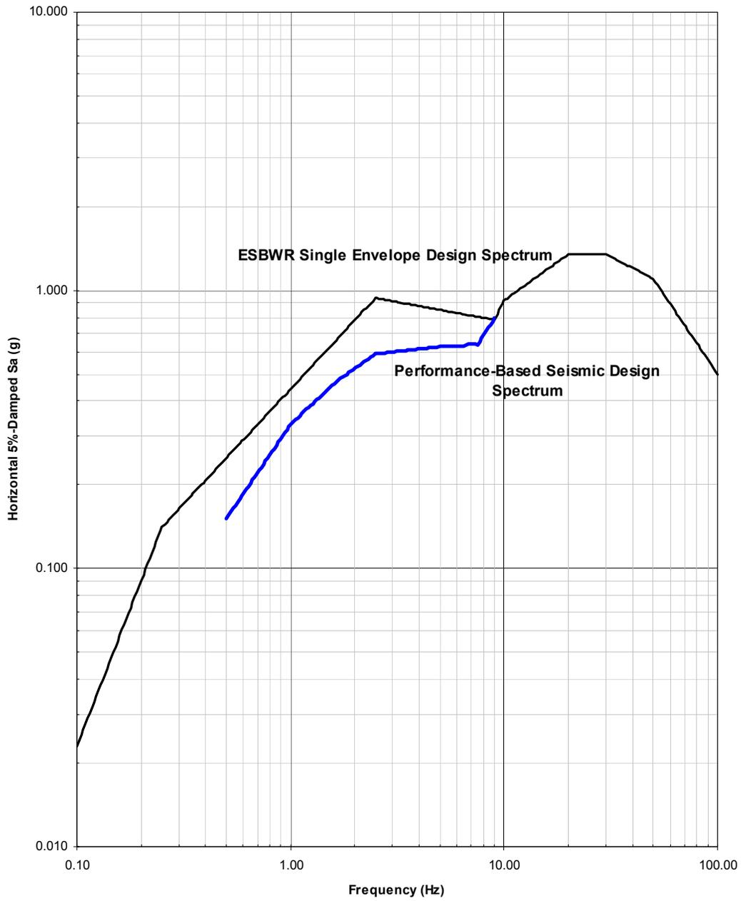
**Figure 15-2. Horizontal Single Envelope Design and Performance-Based Seismic Design Spectra of ESBWR**
