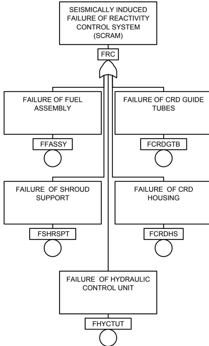
**Figure 15-6. SCRAM Seismic Fault Tree**
