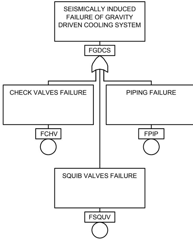
**Figure 15-11. GDCS Seismic Fault Tree**
