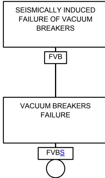
Figure 15-12. VB Seismic Fault Tree
