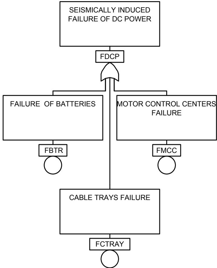
**Figure 15-5. DC Power Seismic Fault Tree**
