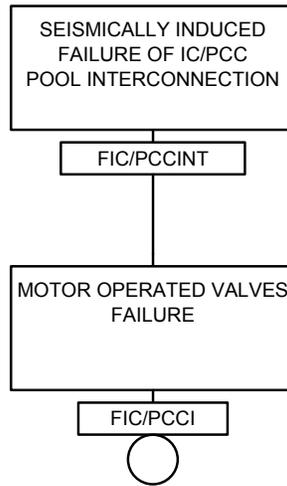
**Figure 15-14. PI Seismic Fault Tree**
