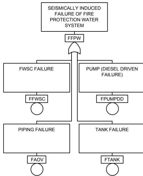
**Figure 15-15. FPW Seismic Fault Tree**
