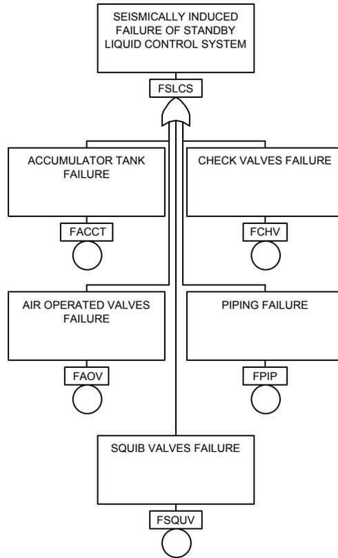
**Figure 15-8. SLCS Seismic Fault Tree**
