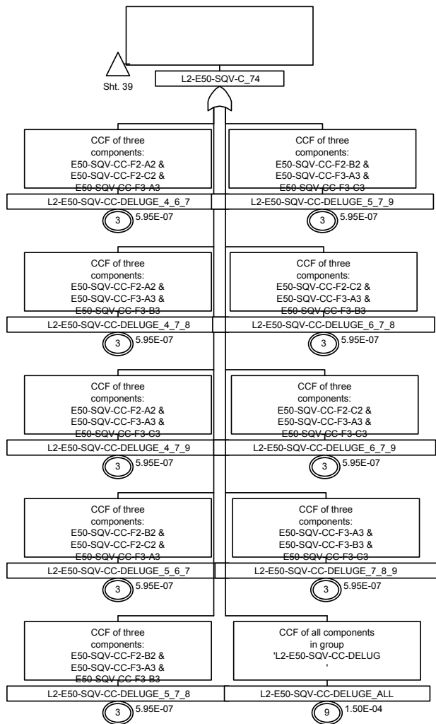
Figure 8A-8. Level 2 Fault Trees
