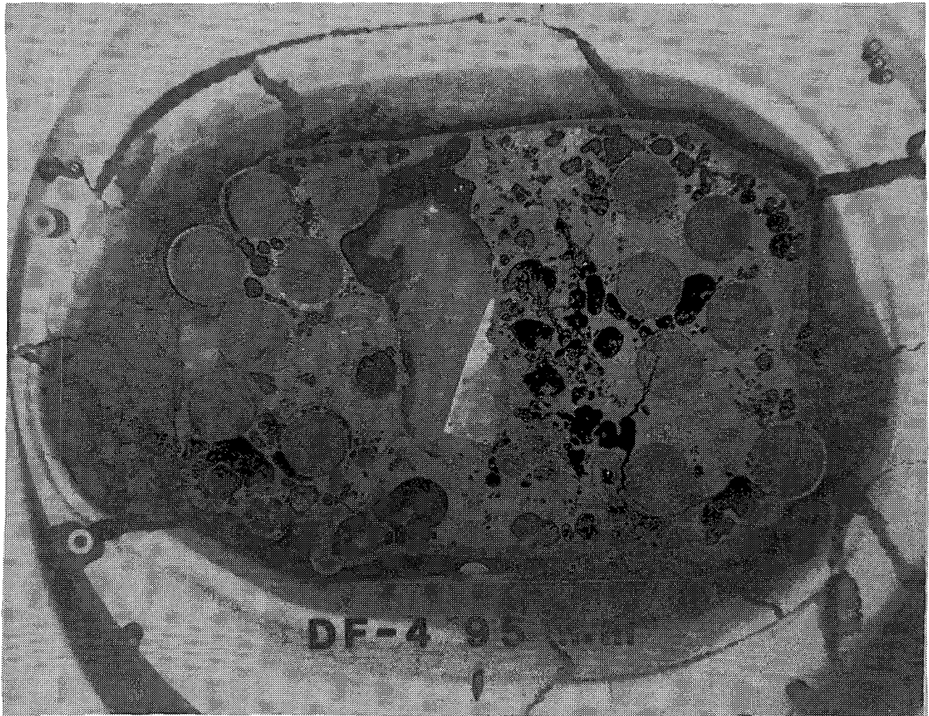
Figure 4.2.11. PIE photo showing final state of the DF-4 test bundle at the 95 mm axial level [5].
