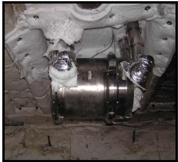
Photograph 8 – Test 2C HAC Thermal Set-up Inside Furnace
