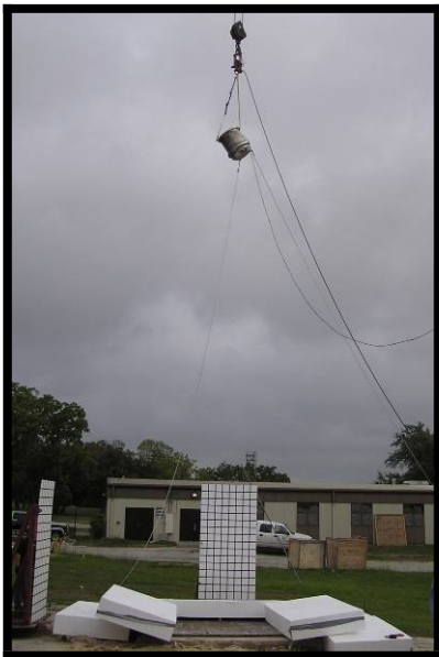
Photograph 3 – Test 1C HAC CG-Over-Top Corner Drop Set-up
