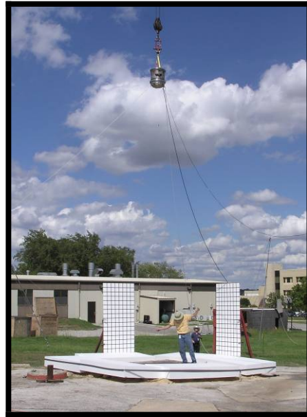
Photograph 2 – Test 1B HAC Top End Drop Set-up
