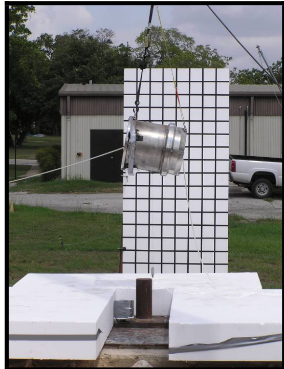
Photograph 6 – Test 2B HAC Side Puncture Drop Set-up
