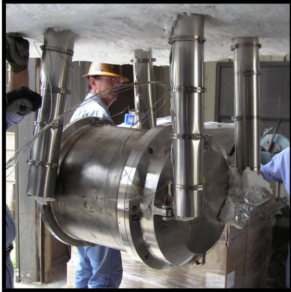
Photograph 7 – Test 2C HAC Thermal Set-up Outside Furnace
