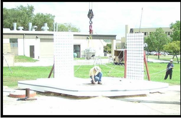
Photograph 1 – Test 1A NCT Bottom End Drop Set-up
