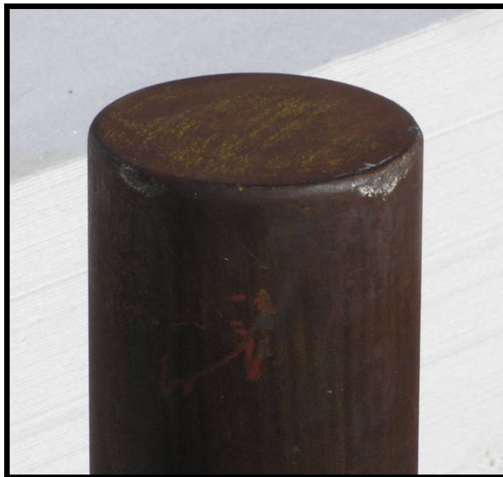
Photograph 18 – Test 1D Puncture Pin Post-Drop Condition (View 2)
