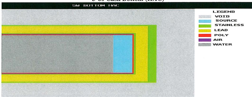
The properties of the shield materials are given in Table 5.1. The stainless steel of the contents is assumed to be Type 316 with densities for the various configurations as given in 5.3.1.
