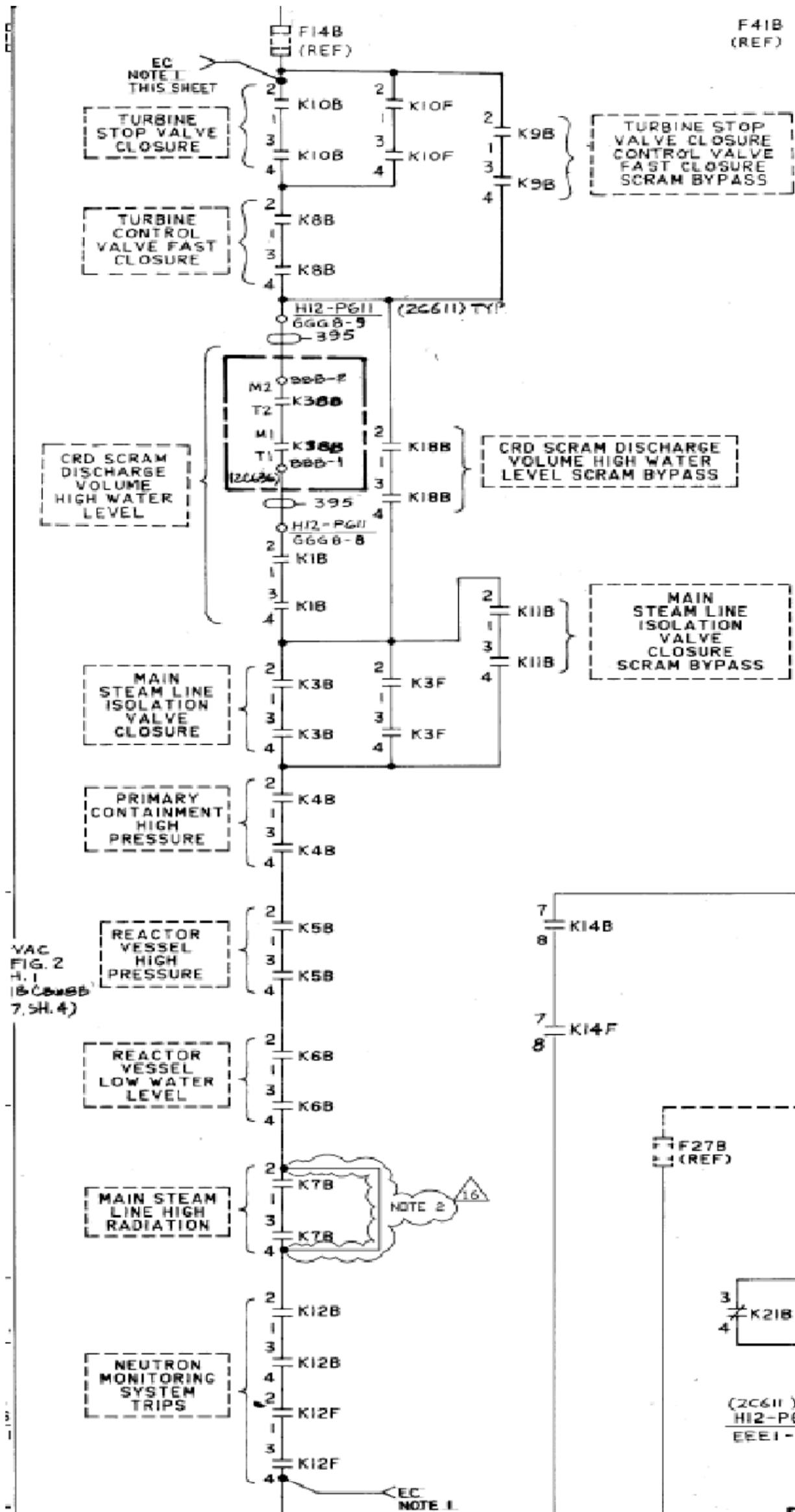
**Figure 4- Balance of Auto-Scrum Circuitry - (typical of 4 Trip Channels)**
