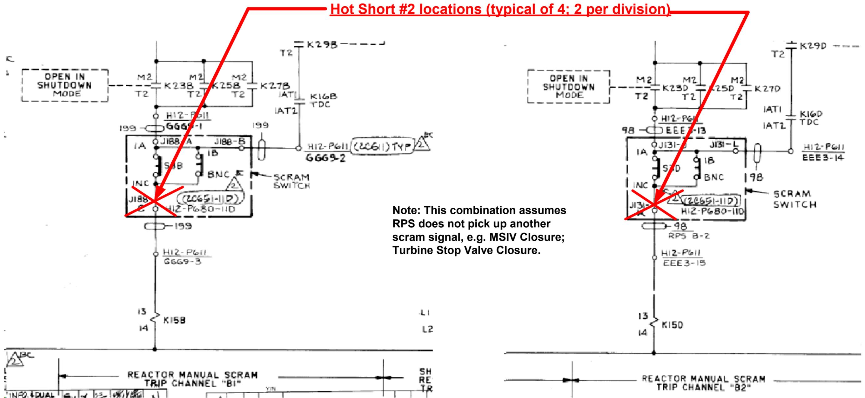
**Figure 2 - Manual Scram Circuitry - Typical of two Trip Systems**
