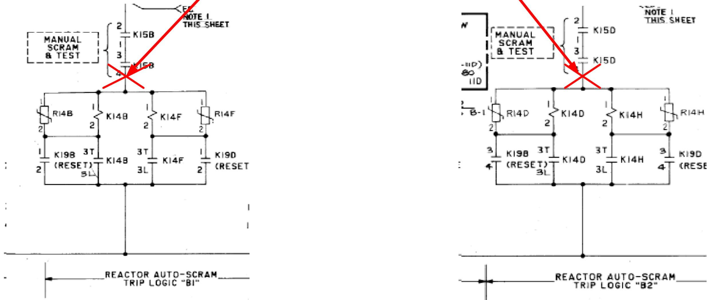
Figure 3 - Reactor Auto-Scram Circuitry - Typical of four Trip
