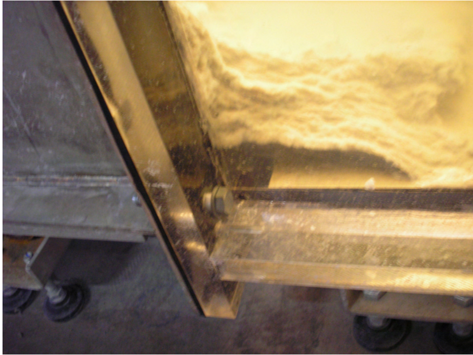
Figure 7 – Upstream View of Apparent Flow Path Under Debris Bed-Salem
