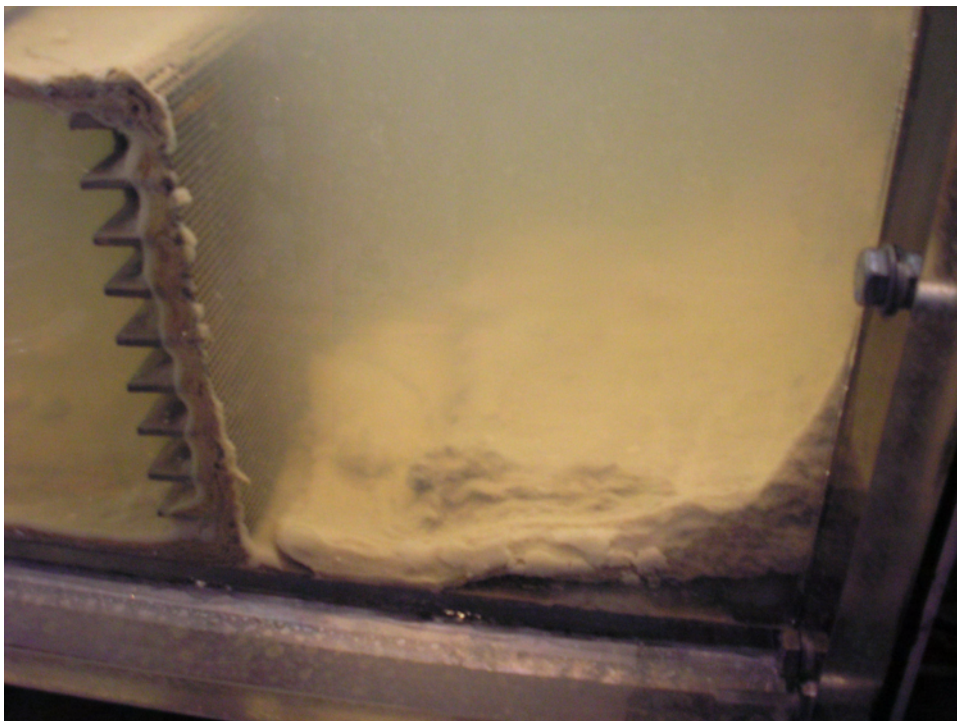
Figure 4 - Fluffy Bed Compressed Following Chemical Addition
