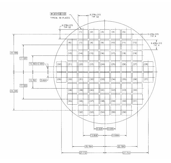
Figure B2-2 BWR Basket Fuel Loading Positions and Minimum Flux Trap Definition
