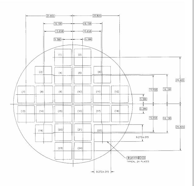
Figure B2-1 PWR Basket Fuel Loading Positions and Minimum Flux Trap Definition
