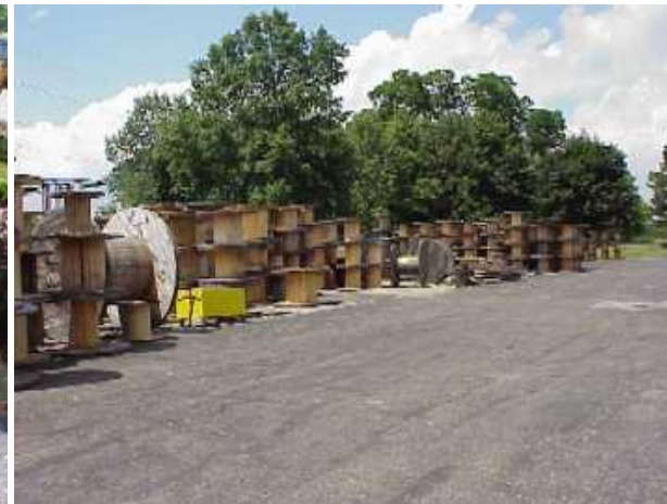
ABOVE: Plastic and wooden spools used to store electrical wire. We started to replace wooden spools with plastic ones that can be used 200 times, versus wooden spools that can be used only about two or three times.
