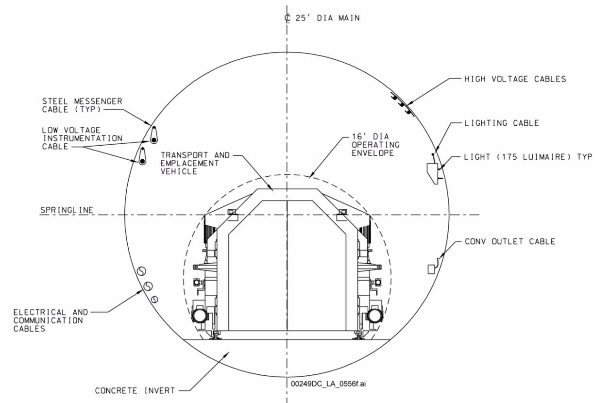
Figure 1.3.3-12. Typical Access Main Finished Cross Section
