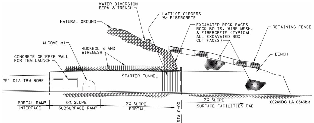
Figure 1.3.3-5. North Portal Long Section with Construction Features
