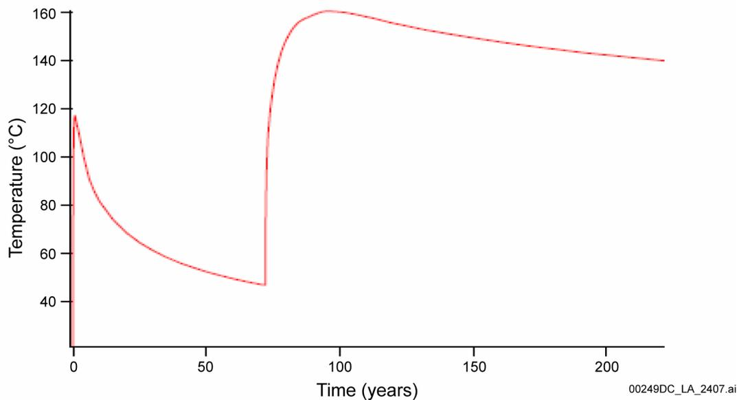
Figure 1.3.1-7. ANSYS Model Results for Warmest Emplacement Drift
