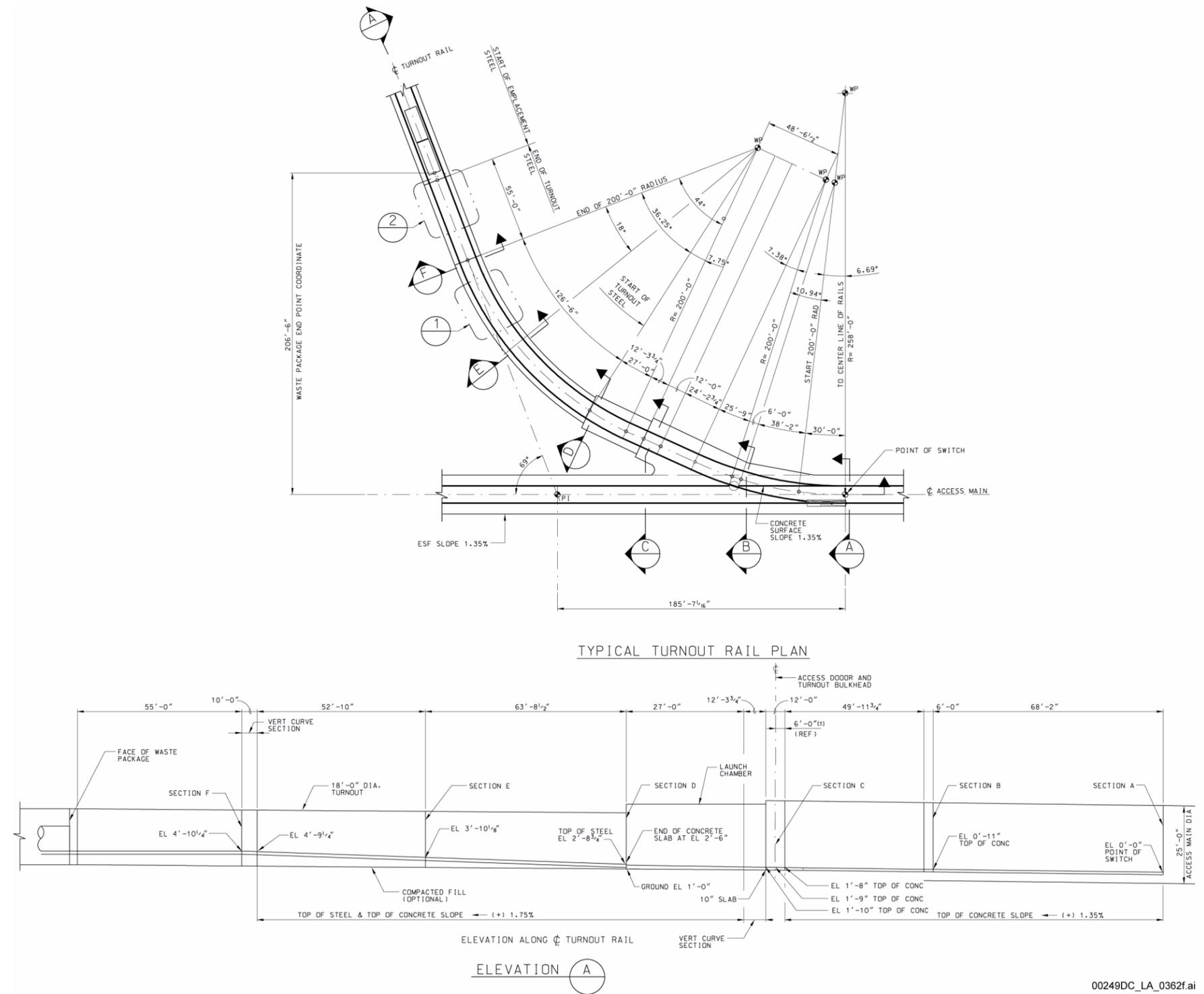
NOTE: 69° angle shown in this figure defines the emplacement drift alignment relative to the alignment of the access main, for a typical turnout configuration in Panels 1 and 2, and it is not the emplacement drift azimuth.
