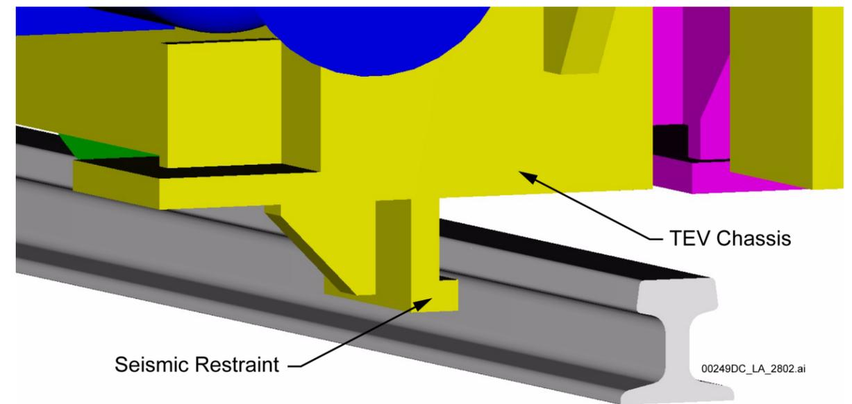
Figure 1.3.3-41. Transport and Emplacement Vehicle Seismic Restraints
