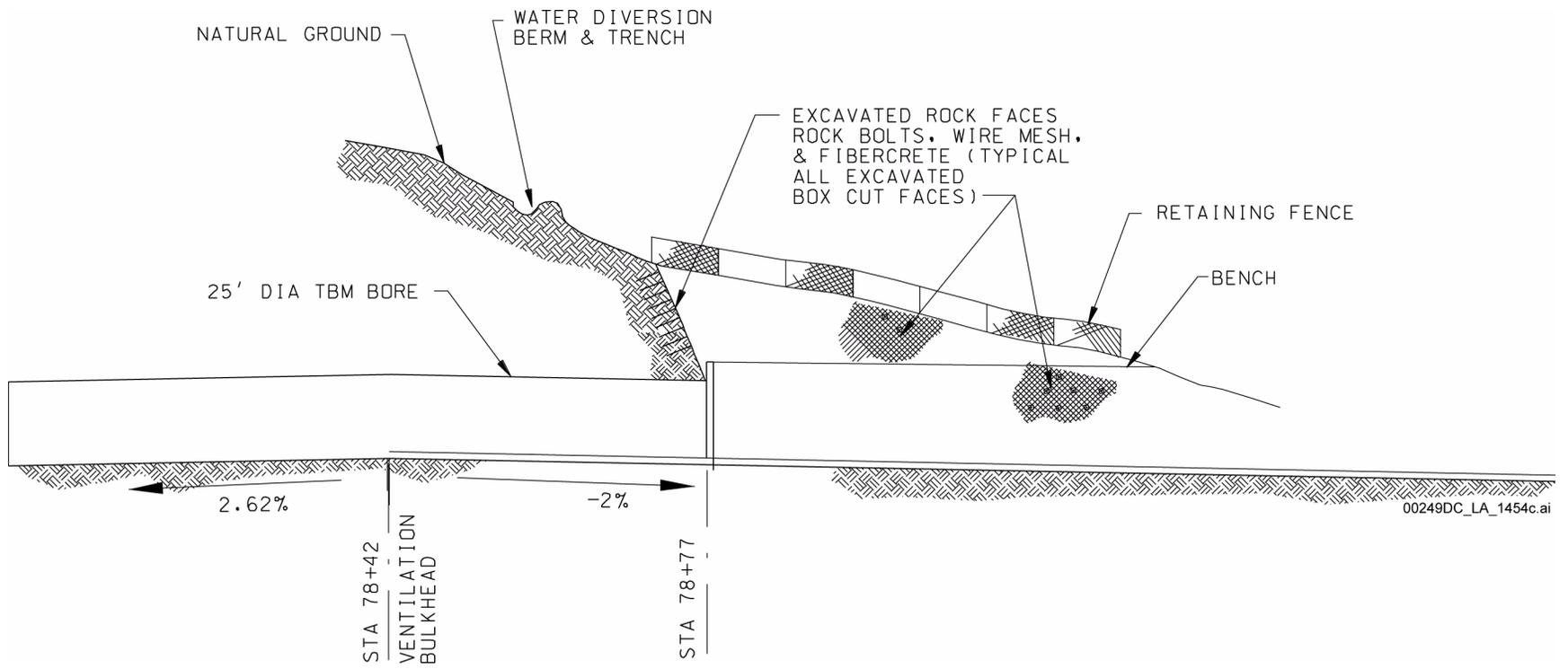
Figure 1.3.3-6. South Portal Long Section with Construction Features
