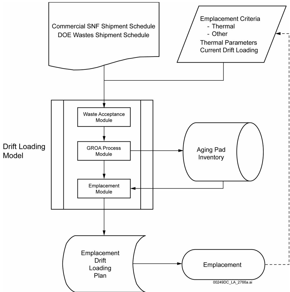
Figure 1.3.1-10. Representation of Emplacement Drift Loading Model
