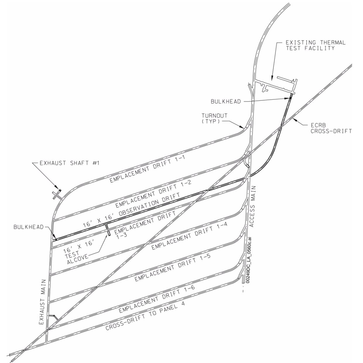
Figure 1.3.3-18. Observation Drift and Test Alcove Plan View
