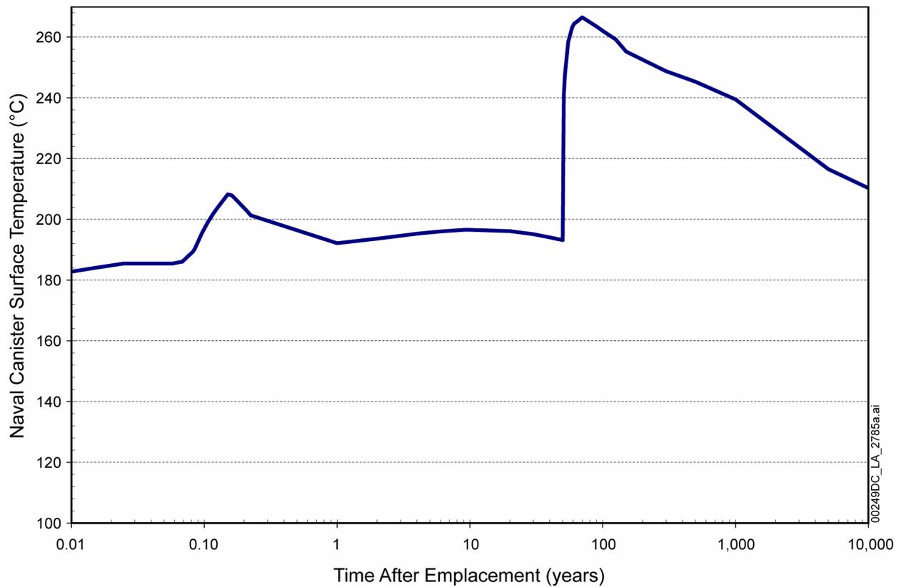
Figure 1.3.1-8. Thermal Envelope for Naval SNF Canister Surface Temperature in Emplacement Drift (Preclosure and Postclosure)
