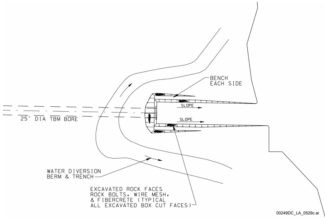
Figure 1.3.3-3. North Construction Portal Plan View (Typical)
