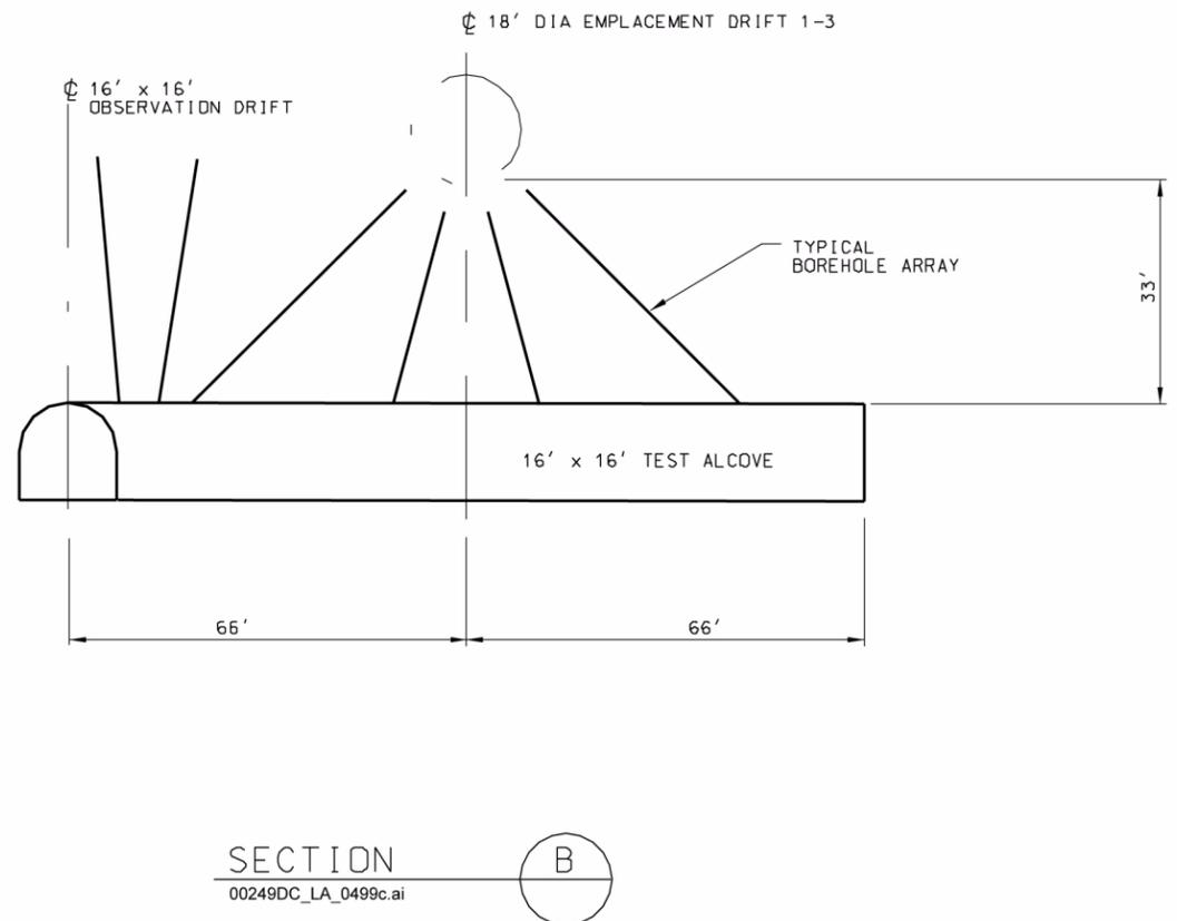
Figure 1.3.3-19. Profile of Observation Drift and Typical Arrangement of Monitoring Boreholes from Observation Alcove
