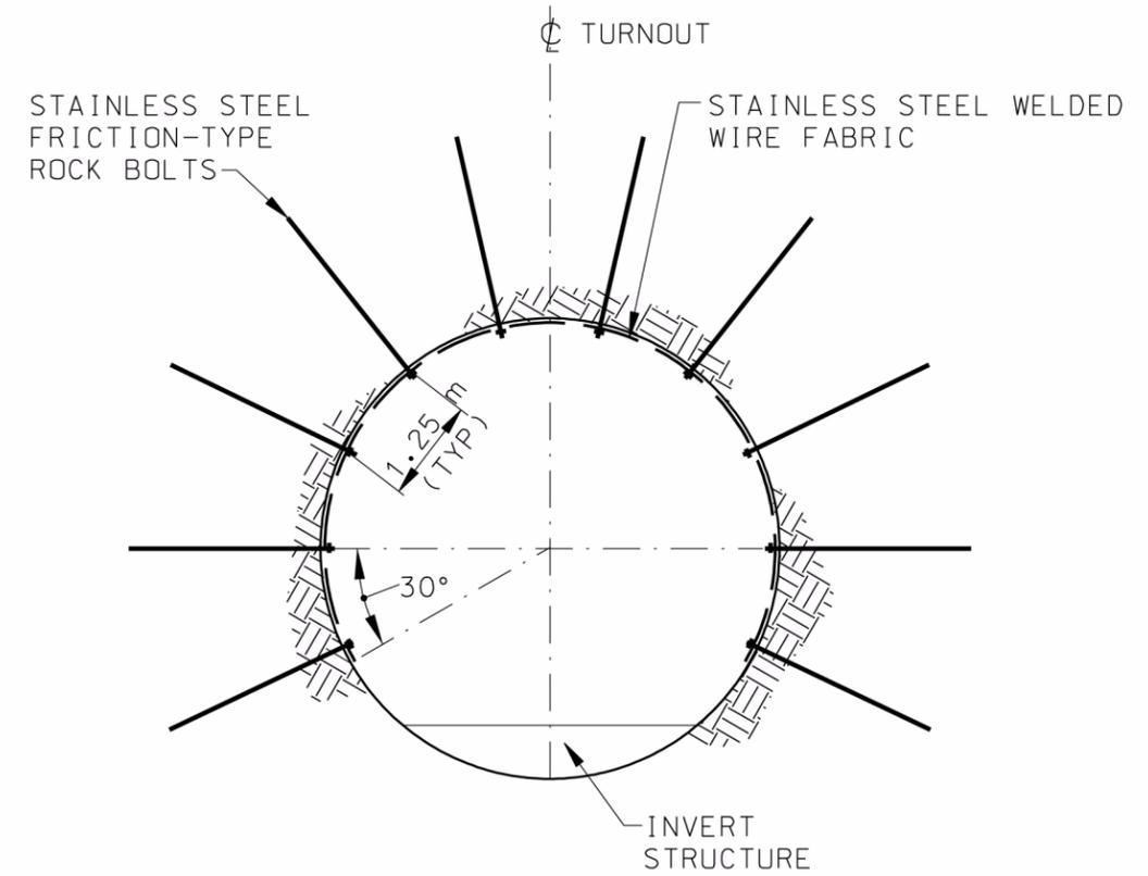
GROUND SUPPORT SYSTEM IN CIRCULAR SECTIONS OF THE TURNOUTS
