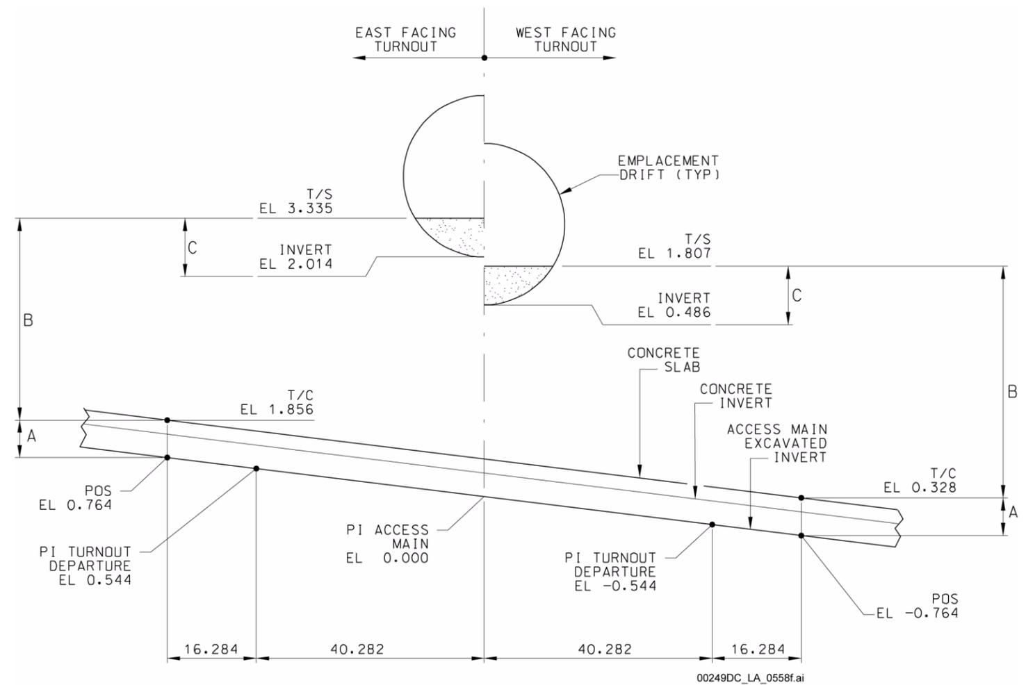
NOTE: Units shown are in meters. PI = point of intersection; POS = point of switch; T/C = top of concrete; T/S = top of steel.
