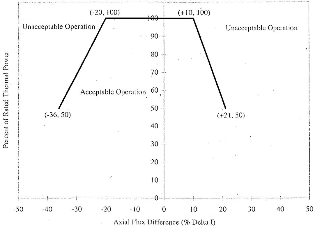
**NOTE:** Compliance with Technical Specification 3.2.1 may require more restrictive AFD limits. Refer to the Unit 1 ROD manual for operational AFD limits.
