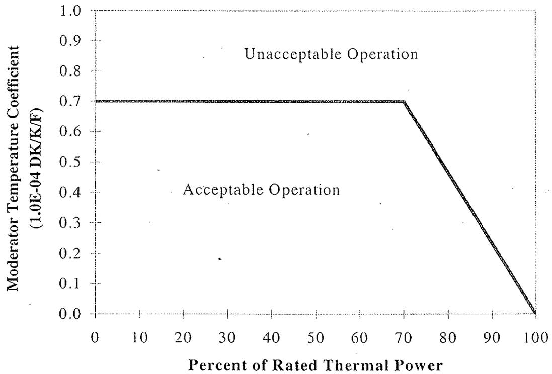
**NOTE:** Compliance with Technical Specification 3.1.3 may require rod withdrawal limits. Refer to the Unit 1 ROD manual for details.
