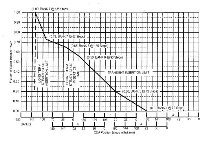
Note: Regulating CEAs that are ≥ 176 steps withdrawn are considered fully withdrawn and are acceptable per this figure.
