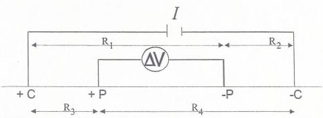
Figure 1: The generalized form of the four electrode array
