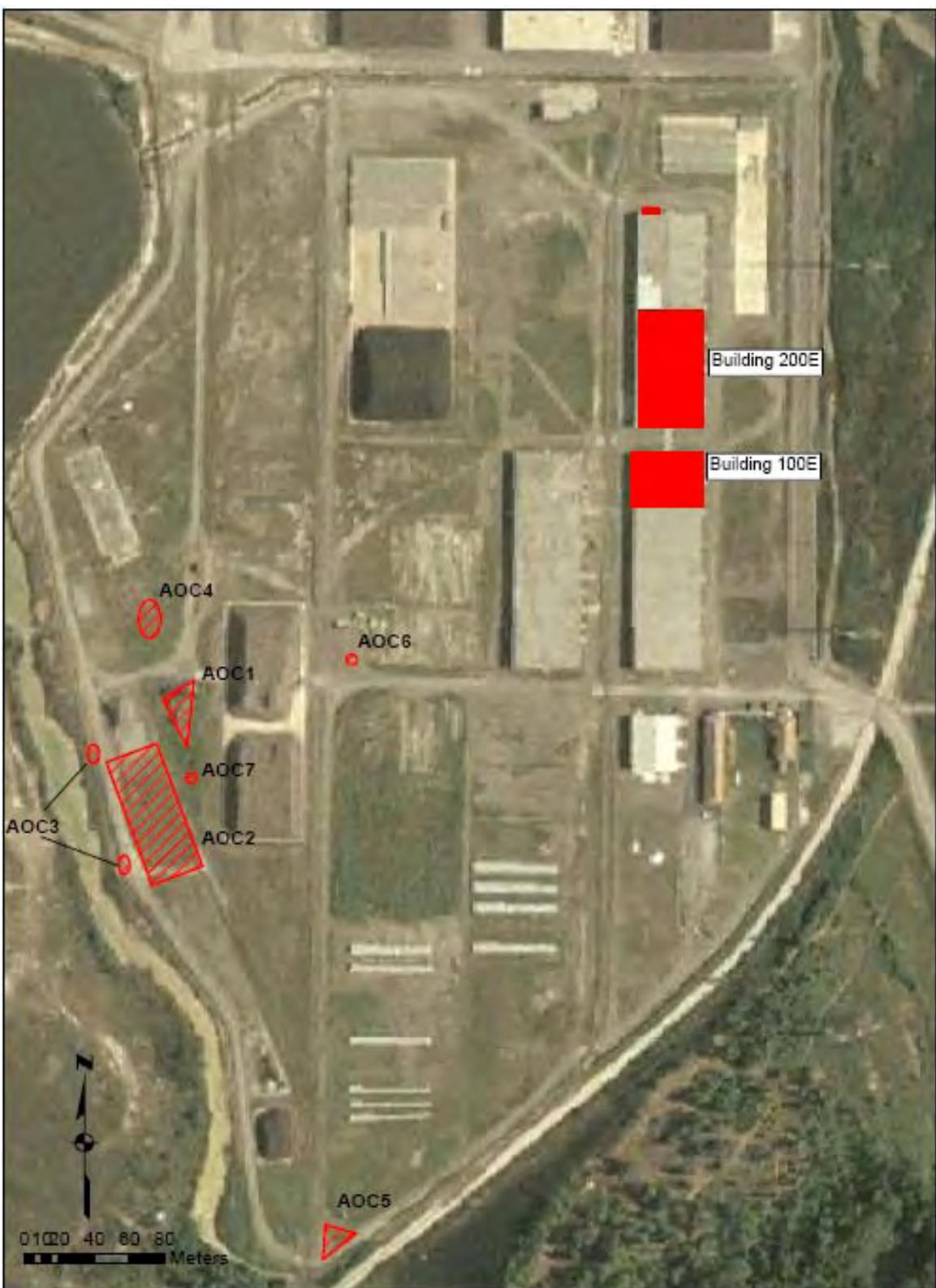
**Figure A-2:** Hammond Depot—Contaminated Buildings and Soil AOCs
