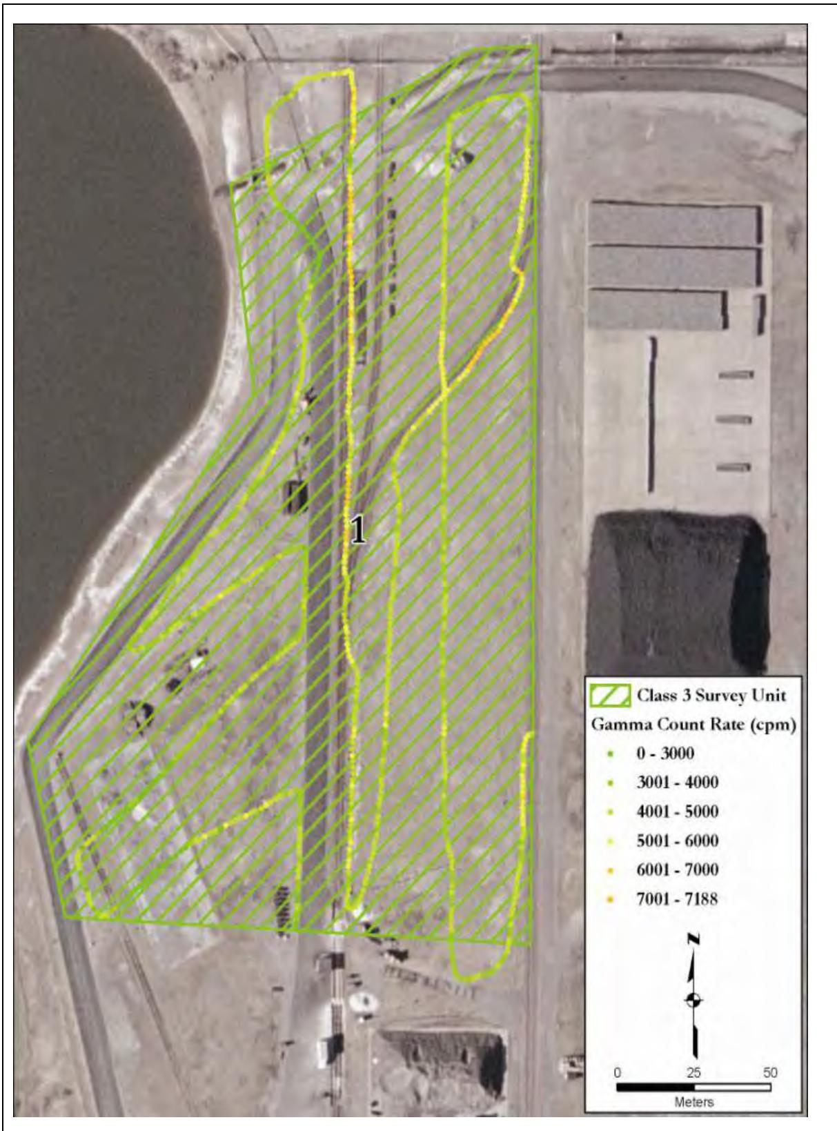
**Figure A-62:** Survey Unit C3 SU1—FSS Gamma Scan Results
