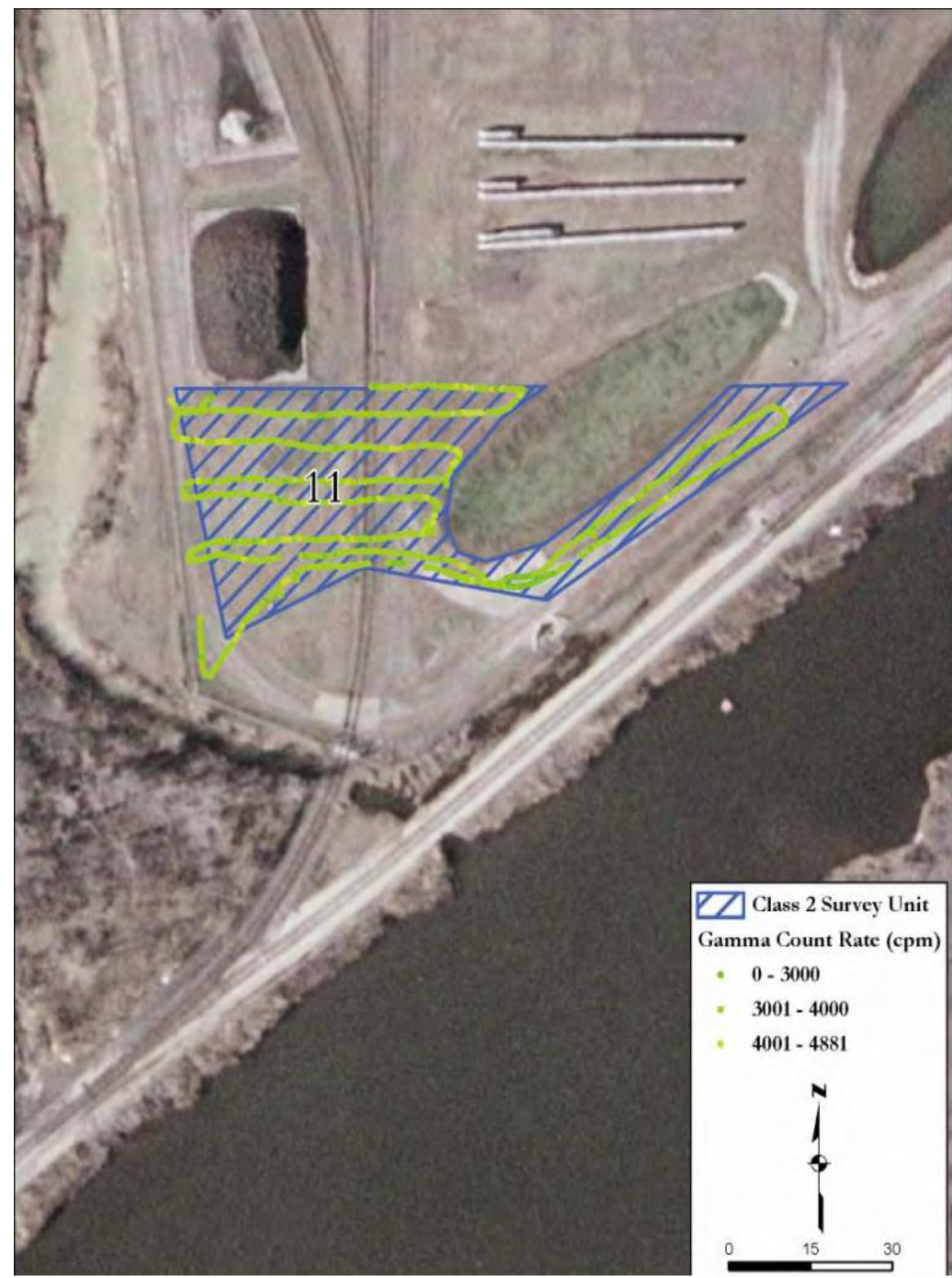
**Figure A-58:** Survey Unit C2 SU11—FSS Gamma Scan Results
