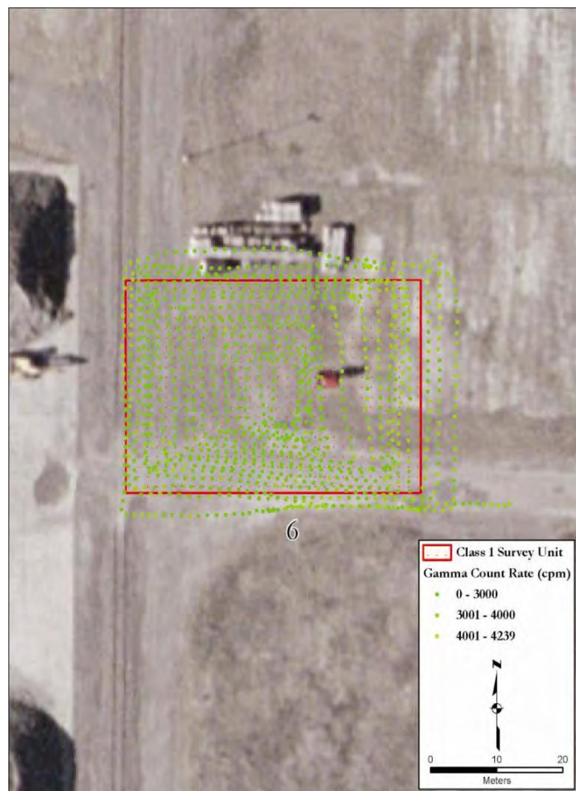
**Figure A-32:** Survey Unit C1 SU6—FSS Gamma Scan Results
