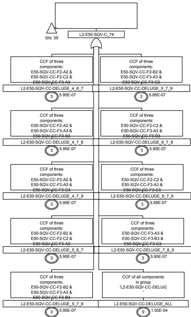
Figure 8A-8. Level 2 Fault Trees
