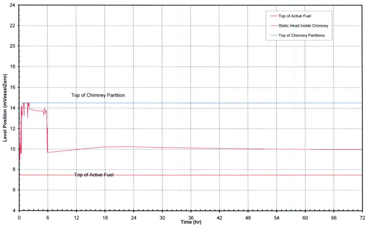
**Figure 6.3-64 S01-1. GDCS Line Break (Bounding Case) – Chimney Collapsed Level (72 hours)**
