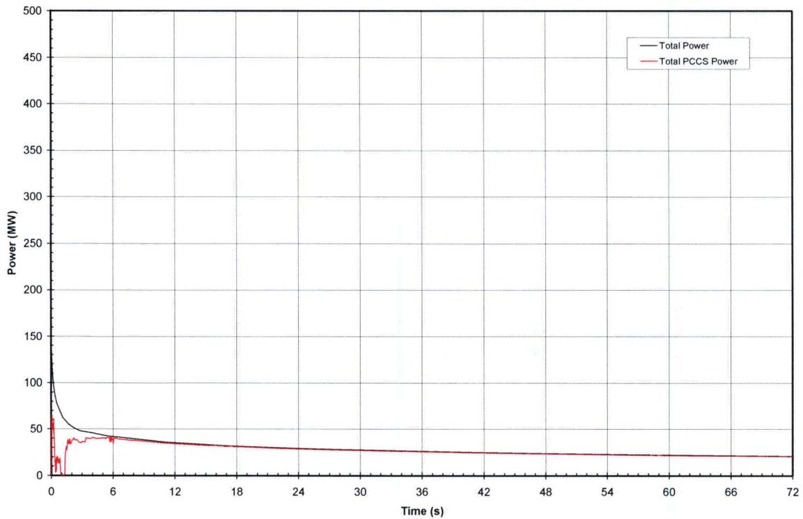
**Figure 6.3-64 S01-2. GDCS Line Break (Bounding Case) – PCCS Heat Removal (72 hours)**
