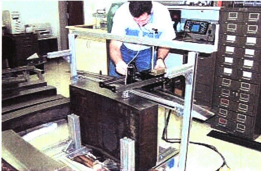
**Figure 3.1 Hope Creek Unit 2 Base Metal Specimen in the NDE Laboratory for Ultrasonic Inspection Using Cut and Machined Surface**
