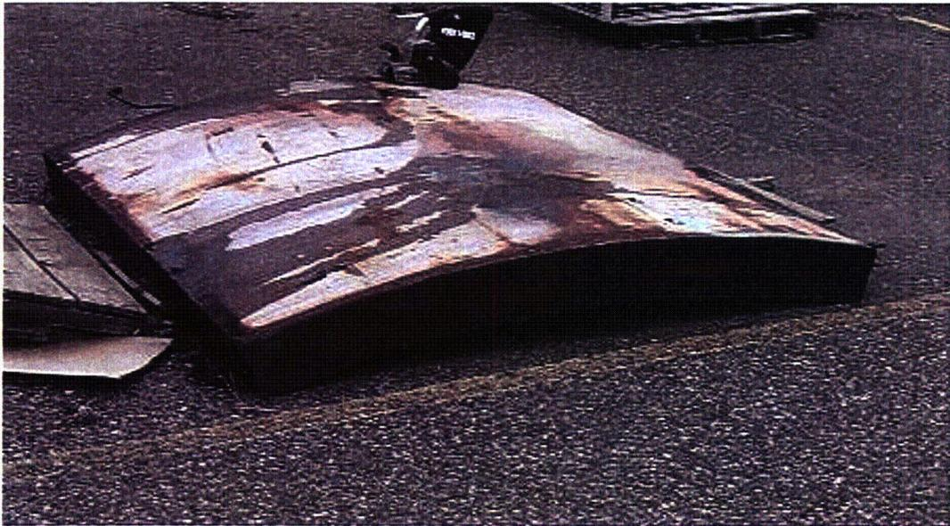
**Figure 3.8 PNNL Reactor Pressure Vessel Specimen as Received from Hope Creek Unit 2**
