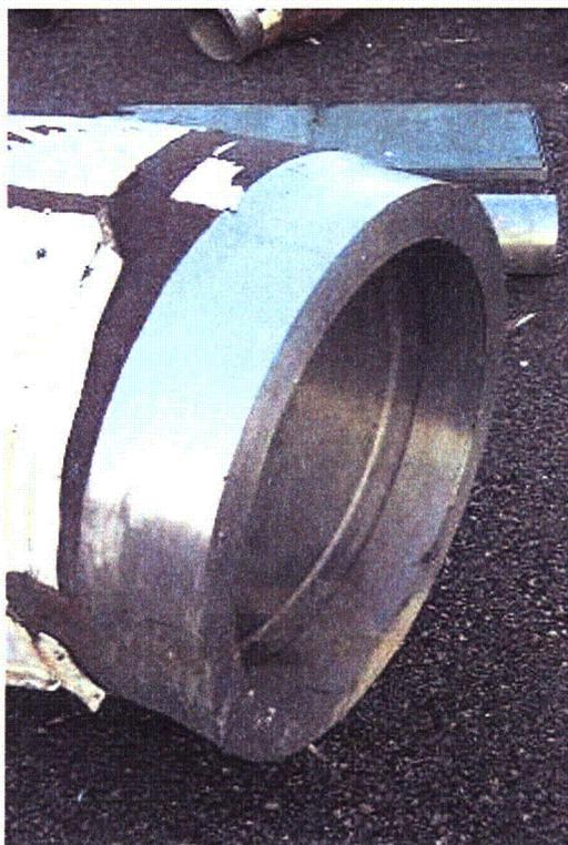
**Figure 3.10 Dissimilar Metal Weld Specimen at PNNL – Safe End to 91-cm-Diameter Carbon Steel Elbow Weld**
