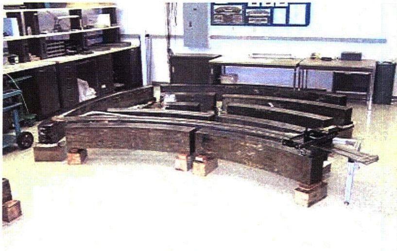
**Figure 3.6 Shoreham Specimens in the PNNL NDE Laboratory, Prepared for Weld-Normal Inspection**
