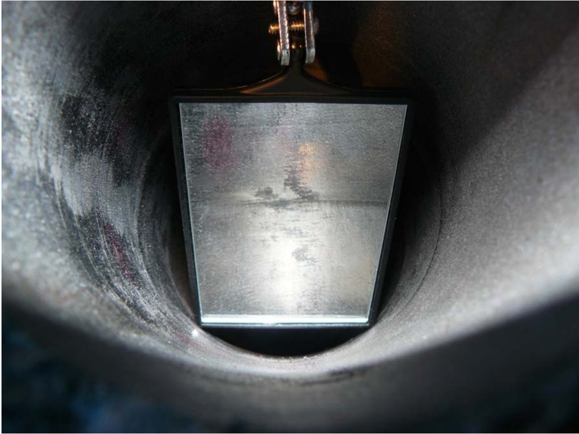
Figure 8: Picture of Nozzle “A” interior. The faint circumferential line in upper portion of the mirror image appears to be the transition between the SS pipe and the alloy 182 weld. The lower circumferential line appears to be from a slight mismatch between the original counterbore machined from the PZR head side and the final post welding machining done from the nozzle flange side. Both of these lines are clearly evident in the eddy current C scan images.
