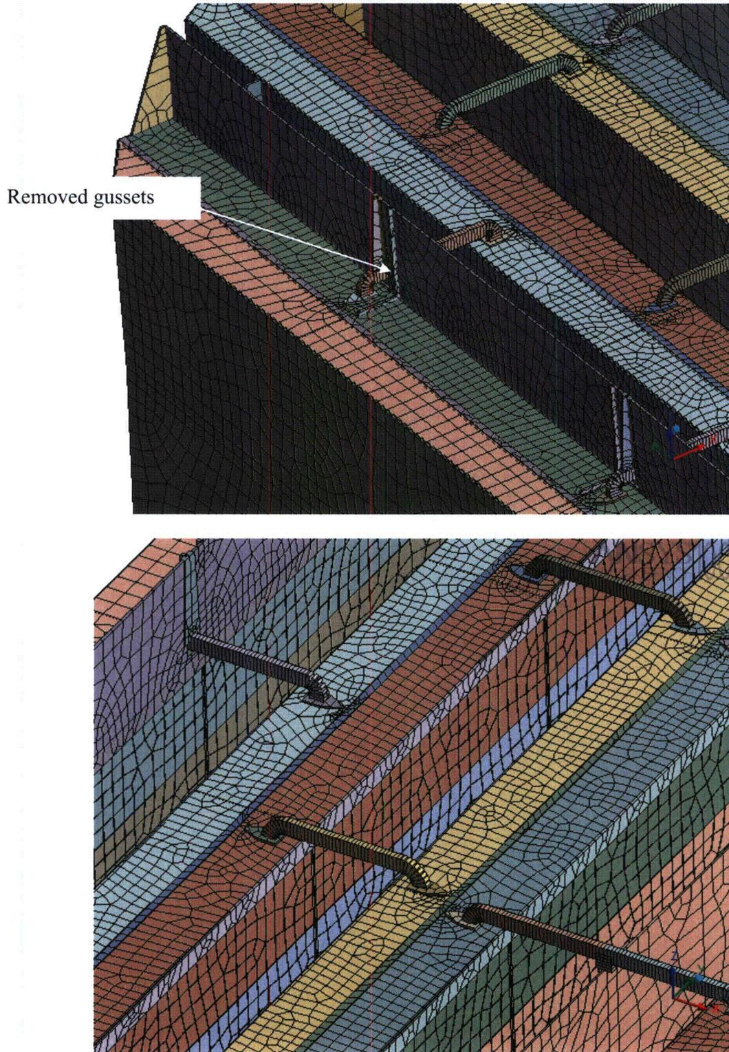
Figure 5f. Close up view of tie bars connecting vane cover plates and adjacent to the steam dam.
