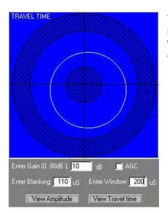
The unhatched ring between the two cross hatched zones represents the sample window. The width of this ring will vary with window length value. The profile of a cylinder is represented here appearing as a circle in the sample window.
