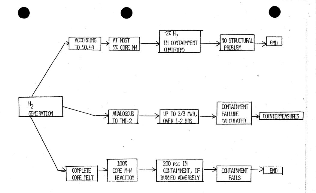
ADIABATIC CONTAINMENT HYDROGEN COMBUSTION CALCULATION
