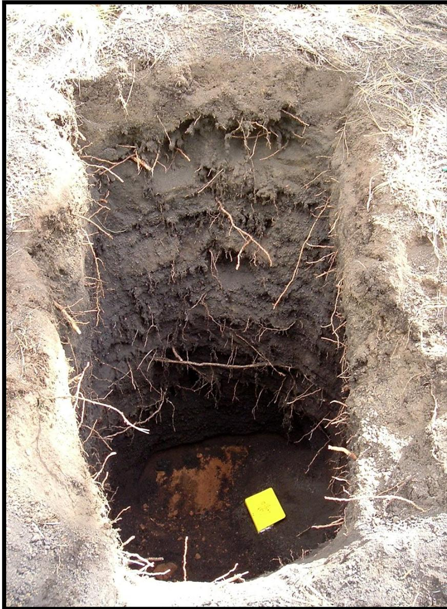
**Figure 2-7. Tephra Pit V30 N6B on Scoria Cone V30 Located South-Southwest of Sunset Crater. Loose Surface Soil and Some Colluvium Obscure Portions of the Pit Walls. Pit Depth is 194 cm [76.4 in].**
