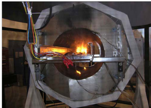
The "small-scale" (Penlight) radiant heating test facility at SNL, shown testing two multi-conductor cables for the US NRC's CAROLFIRE program
