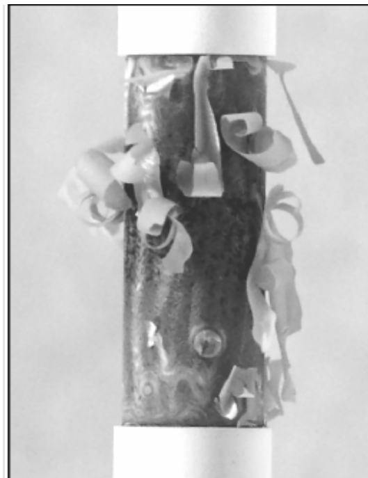
Oxidation of a foreign niobium-bearing cladding alloy under LOCA conditions
