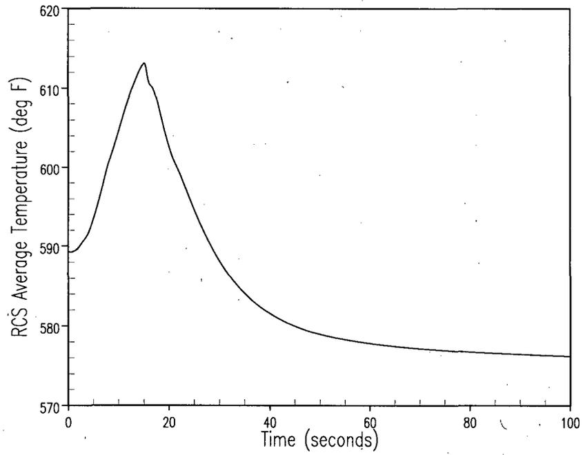
**Figure 2.8.4.2-6 Unit 2 Loss of Load/Turbine Trip RCS Overpressurization Analysis
