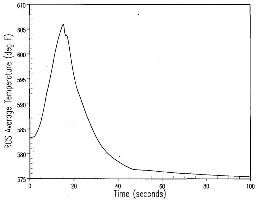
**Figure 2.8.4.2-3 Unit 1 Loss of Load/Turbine Trip RCS Overpressurization Analysis RCS Average Temperature vs. Time**
