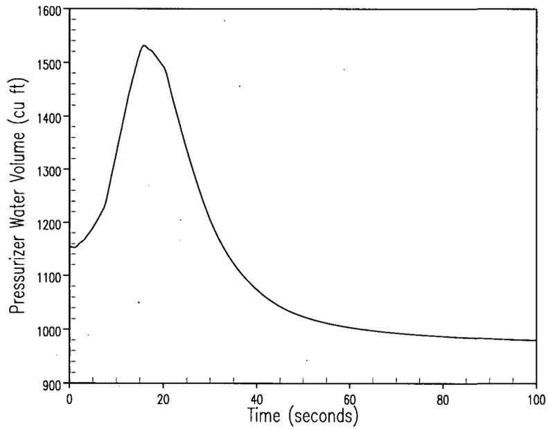
**Figure 2.8.4.2-5 Unit 2 Loss of Load/Turbine Trip RCS Overpressurization Analysis
