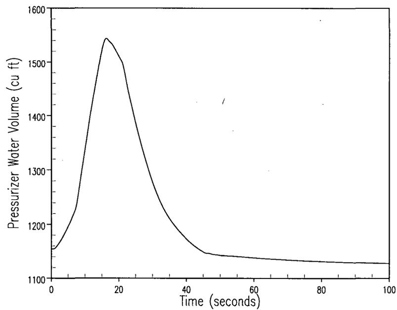
**Figure 2.8.4.2-2 Unit 1 Loss of Load/Turbine Trip RCS Overpressurization Analysis RCS Pressure and Pressurizer Water Volume vs. Time**
