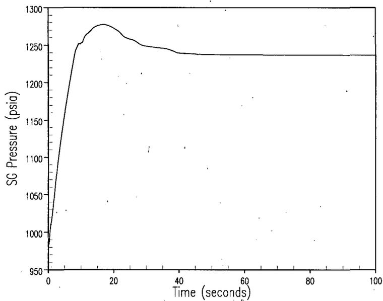
**Figure 2.8.4.2-1 Unit 1 Loss of Load/Turbine Trip RCS Overpressurization Analysis
