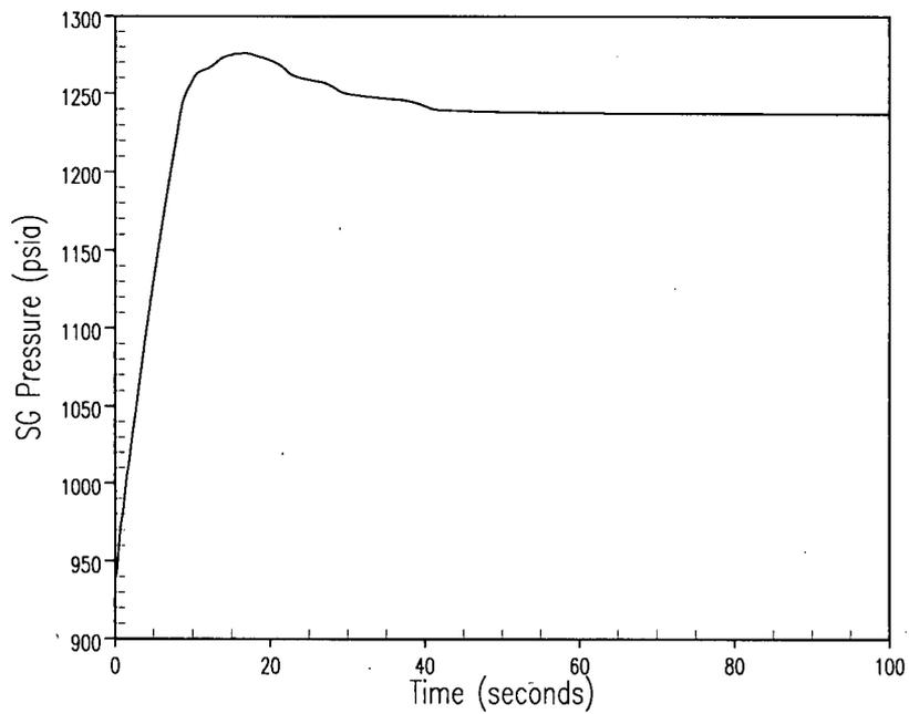
**Figure 2.8.4.2-4 Unit 2 Loss of Load/Turbine Trip RCS Overpressurization Analysis Nuclear Power and Steam Generator Pressure vs. Time**
