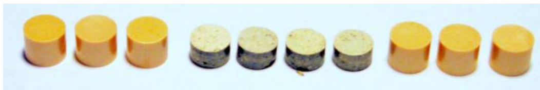
Figure 4.4 Phase 2+ Un-doped and Fission Product-Doped Cerium Oxide Pellets
