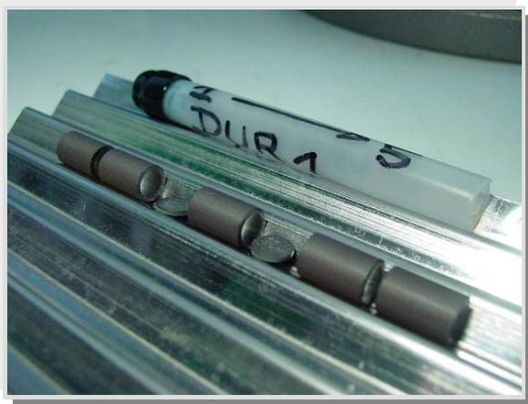
Figure 5.2 DUO<sub>2</sub> Pellets and Dopant Disks for Test 3/1
