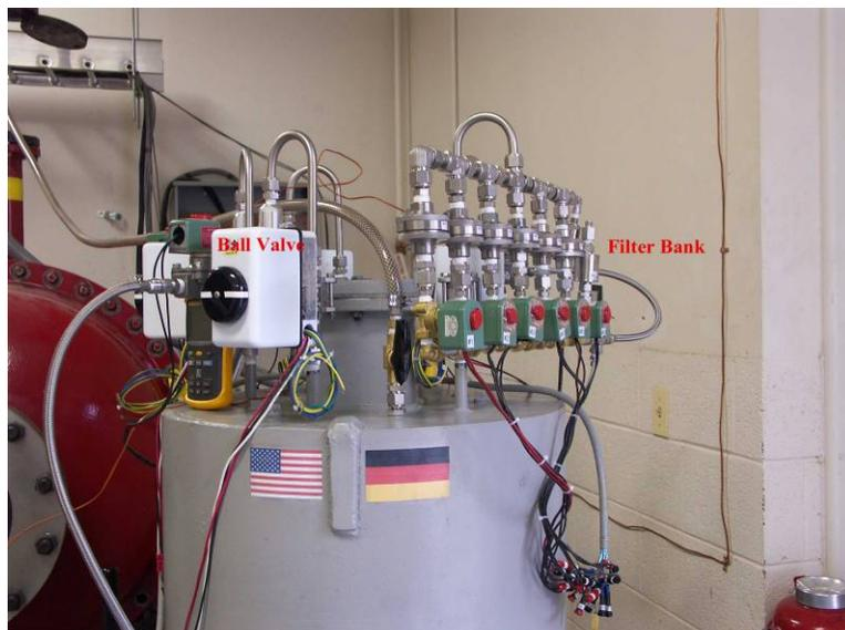
Figure 4.12 Gelman Filter Bank Sequential Samplers
