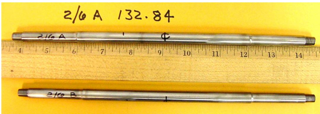
Figure 4.2 Pressurized Test Rodlets for Tests 2/6A and 2/6B
