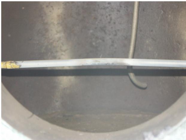
Figure 6.7 Test 2/5F Post-test Rodlet, Bent
