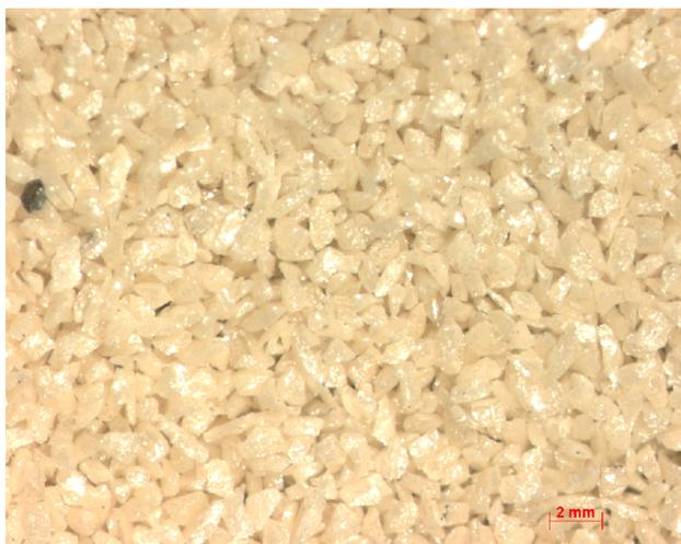
Figure 6.18 Test 2/5G Rod Debris, 100  $\mu\text{m}$  fraction
