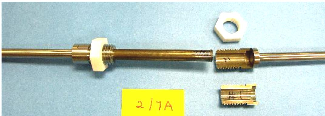
Figure 4.5 German HLW Glass Test Rodlet for Tests 2/7A
