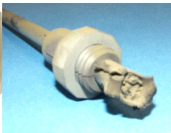
Figure 6.4 Post-test Glass Target Rodlet, Test 2/7A
