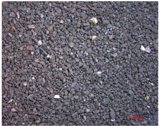
Figure 6.20 Test 2/6A Impact Debris, 250  $\mu\text{m}$  fraction
