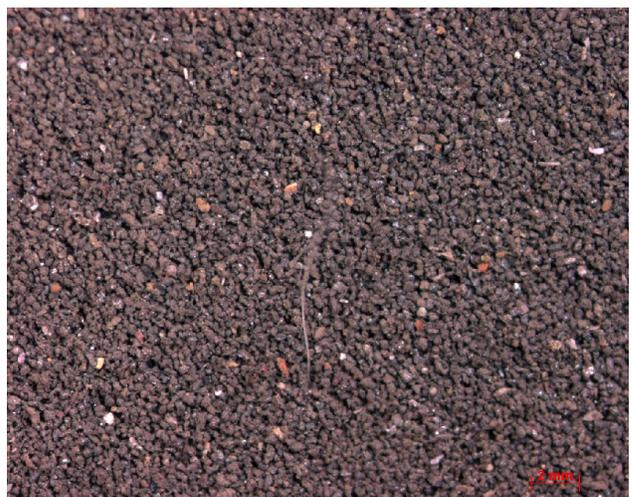
Figure 6.21 Test 2/6A Impact Debris, 74  $\mu\text{m}$  fraction
