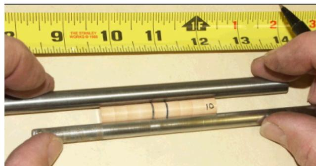
Figure 4.4 Fission Product Dopant Disks, Adjacent to Central Pellet, Test 2/5E
