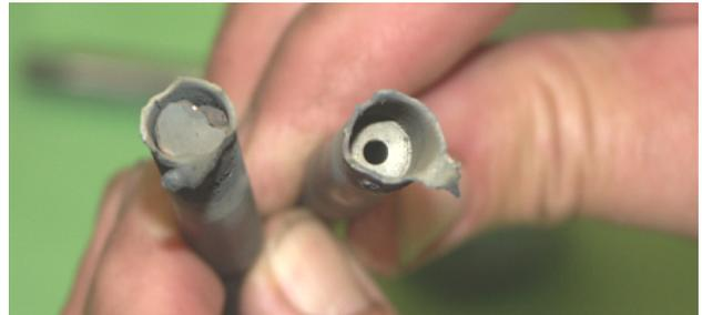
Figure 6.11 Test 2/6A Post-test Rodlet Ends
