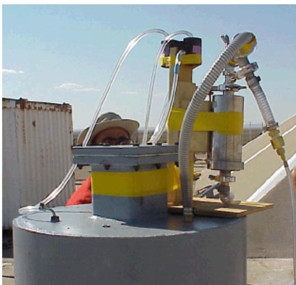
Figure 6.1 Test 2/5A Aerosol Sampling Apparatus
