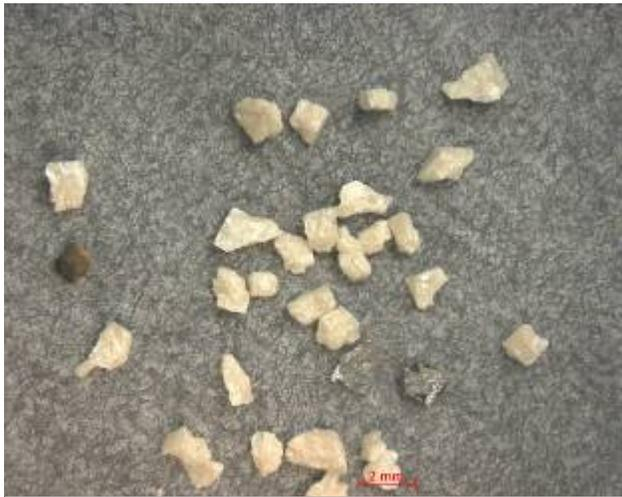
Figure 6.16 Test 2/5G Rod Debris, 500  $\mu\text{m}$  fraction
