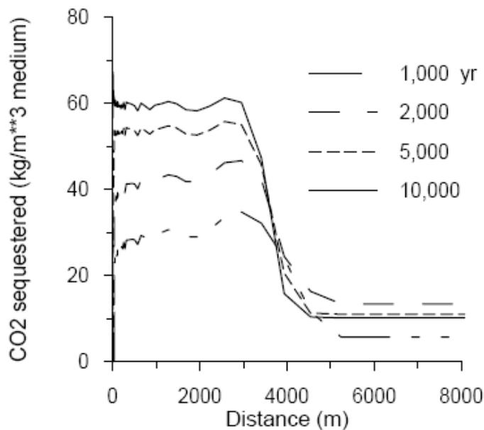
**Figure 6-18. Cumulative CO<sub>2</sub> Sequestration by Carbonate Precipitation for Different Times. The Positive Values in the Background Region ( $x > 4000$  m) are Due to Calcite Precipitation. Figure from Xu, et al., 2005. Results for the Validation and Supplied Output are Shown as One Set of Identical Data.**
