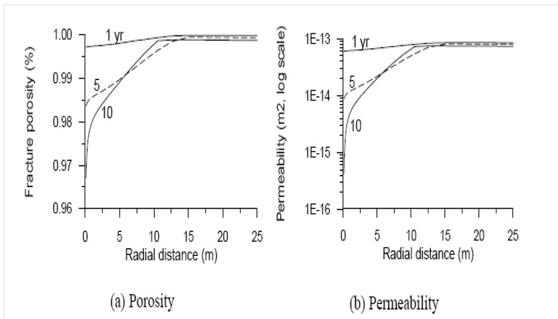
**Figure 6-32. Distribution of Porosity and Permeability along the Well Radius for the Simulation Shown in Figure 6.3.8.4. Figure from Xu, et al., 2005. Results for the Validation and Supplied Output Are Shown as One Set of Identical Data.**
