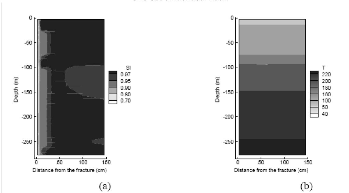
**Figure 6-25. Liquid Saturation (a) and Temperature (b, in °C) in the Fracture-matrix System. This and Subsequent Contour Plots Extend to a Distance of 145 cm [57.09 in], Which Is the Distance Between the Center of the Fracture Zone, and the Nodal Point at the Center of the Innermost Matrix Grid Block. The Overall Size of the Model Domain is 175 cm [68.9 in]. Figure from Xu, et al., 2005. Results for the Validation and Supplied Output Are Shown as One Set of Identical Data.**
