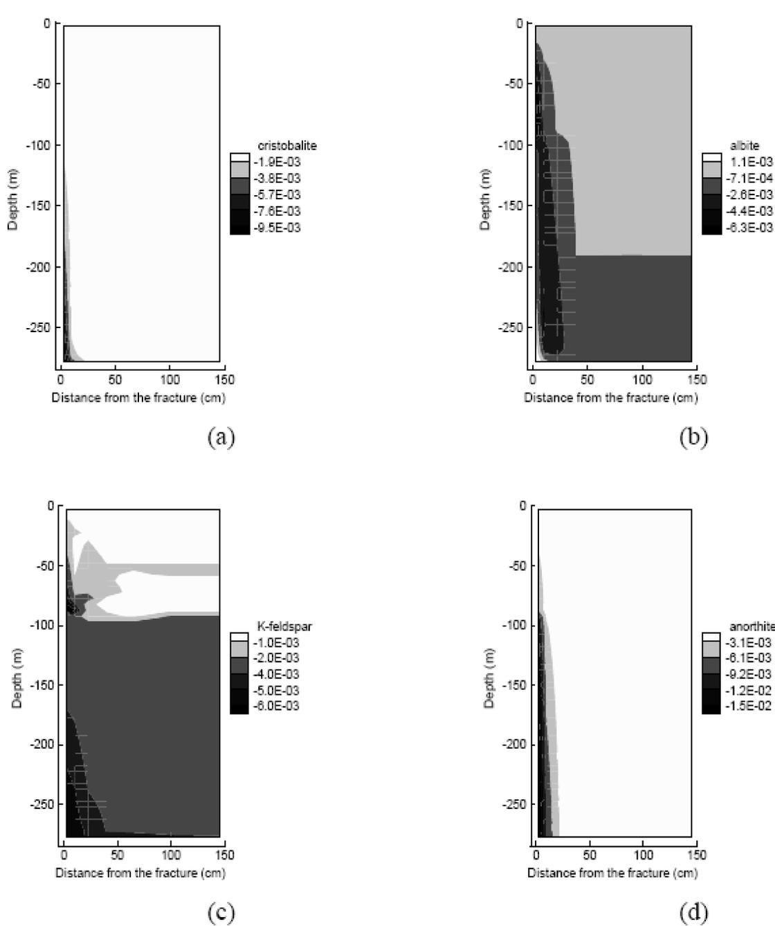
**Figure 6-26. Change of Primary Mineral Abundance (In Volume Fraction) after 1,000 years. The Inflection Points in the Figures Result from (i) Grid Discretization and (ii) Highly Non-Linear Nature of Heterogeneous Reactions. The Space Discretization in the Simulation Is Not Fine Enough to Give an Accurate Definition of Mineral Abundances near Inflection Points. Figure from Xu, et al., 2005. Results for the Validation and Supplied Output Are Shown as One Set of Identical Data.**
