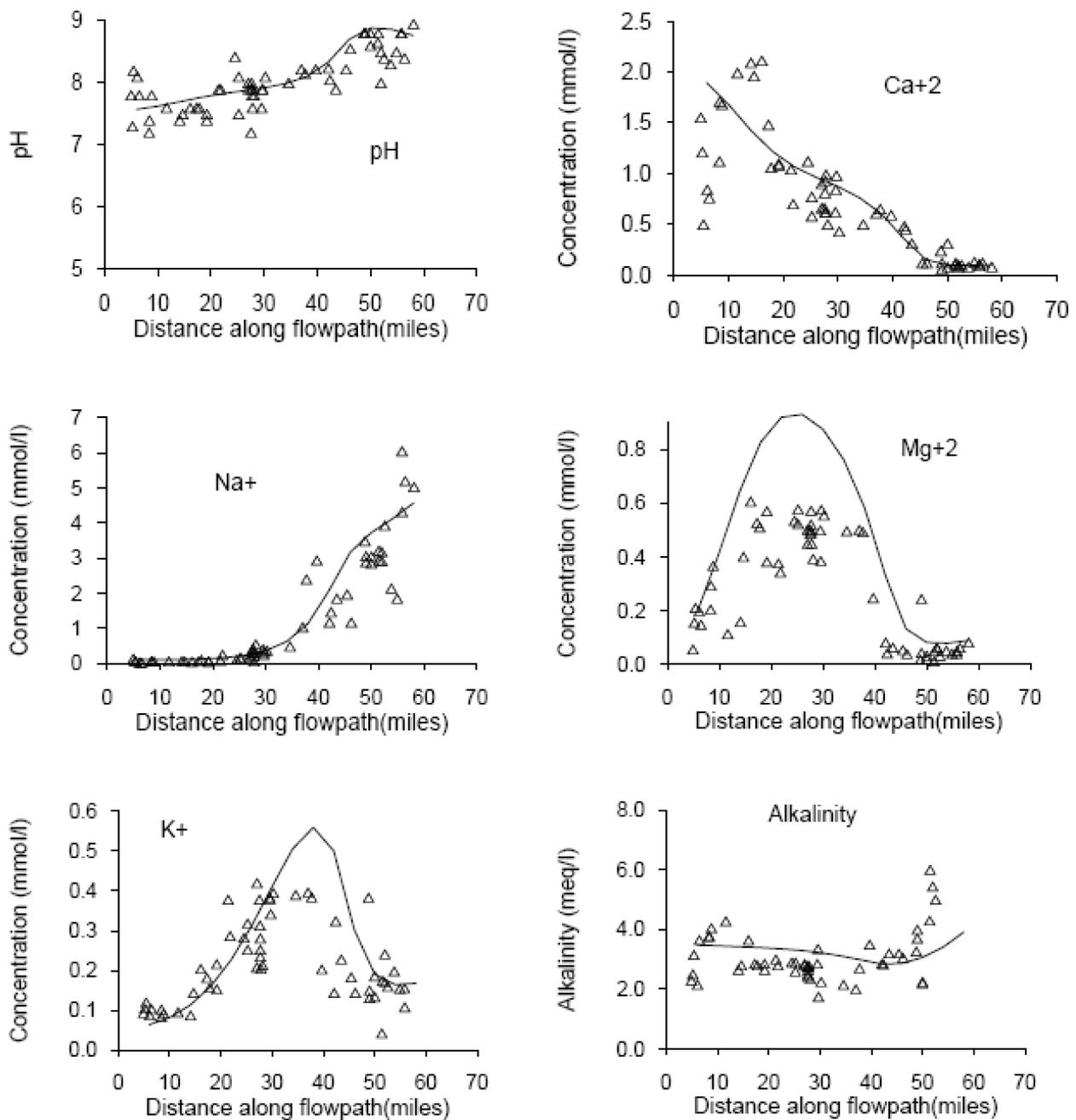
Figure 6-4. Concentrations of  $\text{Na}^+$ ,  $\text{K}^+$ ,  $\text{Mg}^{2+}$ ,  $\text{Ca}^{2+}$ , Alkalinity, and pH Along a Flow Path in the Aquia Aquifer (Maryland). Symbols Indicate Observations Provided by Appelo (1994) and Originally from Chapelle and Knobel (1983); Solid Lines Represent Simulated Concentrations Using TOUGHREACT. Figure from Xu, et al., 2005. Results for the Validation and Supplied Output are Shown as One Set of Identical Data.
