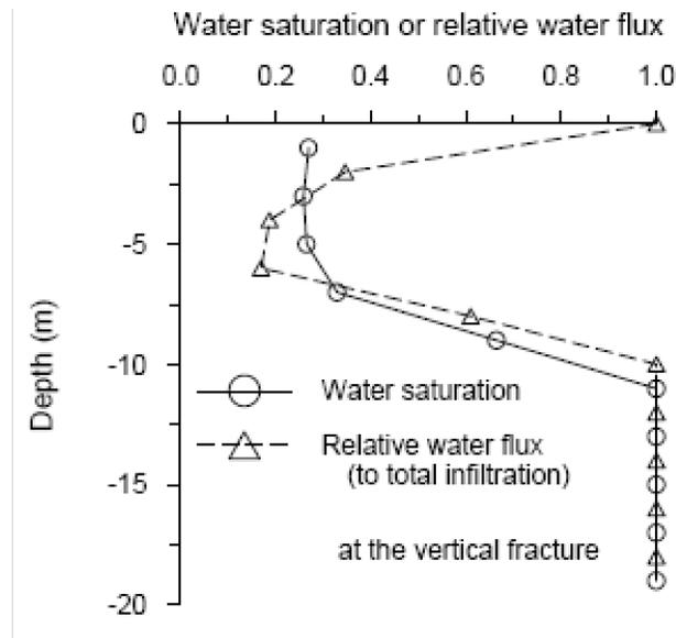
**Figure 6-22. Steady-State Water Saturation and Water Flux (Relative to Total Infiltration) Passed Through the Fractures. Figure from Xu, et al., 2005. Results for the Validation and Supplied Output are Shown as One Set of Identical Data.**
