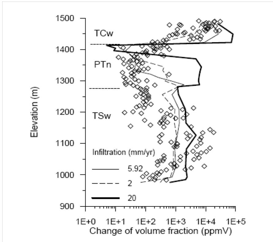
**Figure 6-7. Simulated Total (Fracture Plus Matrix) Calcite Abundances (Volume Fraction) in the WT-24 Column for Different Infiltration Rates after 10 Million Years (Extended Geochemical System). Diamonds Represent Bulk Rock Calcite Abundances Measured by the U.S. Geological Survey (Paces, et al., 2001). Figure from Xu, et al., 2005. Results for the Validation and Supplied Output are Shown as One Set of Identical Data.**
