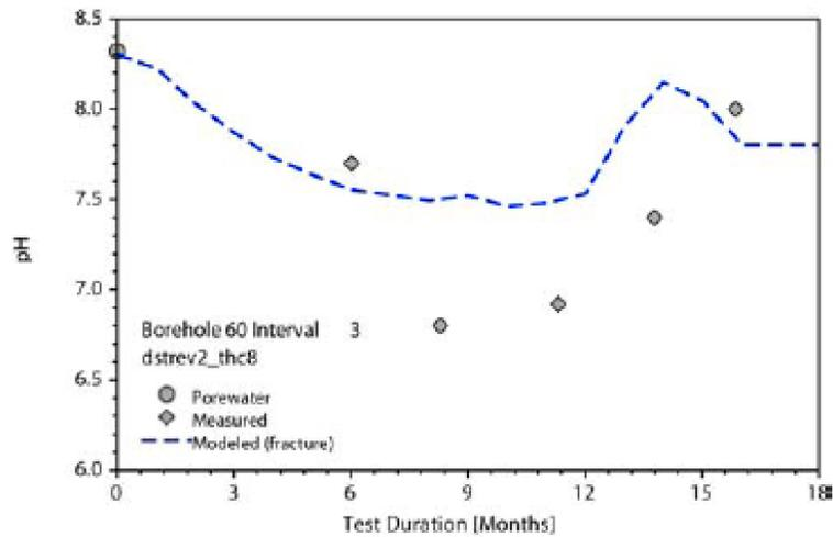
**Figure 6-10. Measured and Modeled pH (in Fractures) for Samples Collected from Borehole Interval 60-3, Located Below the Heaters. Figure from Xu, et al., 2005. Results for the Validation and Supplied Output are Shown as One Set of Identical Data.**
