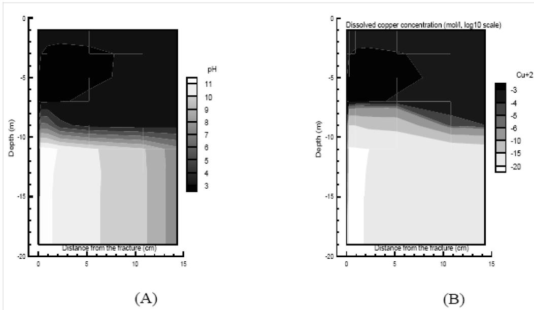
**Figure 6-24. pH and Dissolved Copper Concentration at 20,000 Yrs in the Fractured Rock. Figure from Xu, et Al., 2005. Results for the Validation and Supplied Output Are Shown as One Set of Identical Data.**
