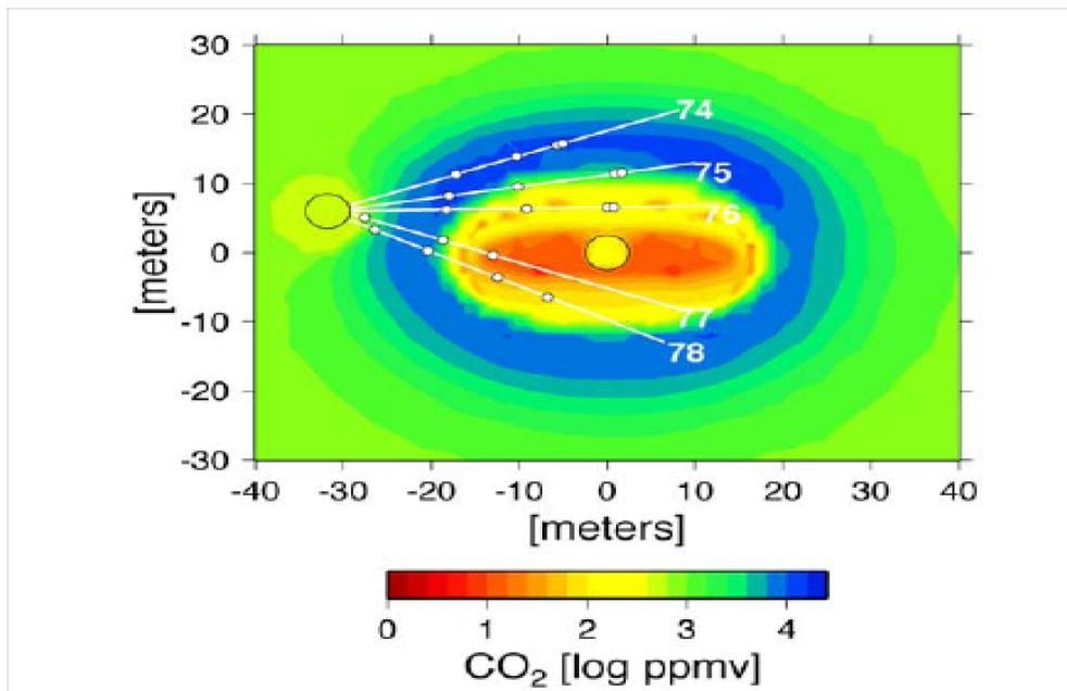
**Figure 6-11. Borehole Positions. Modeled Gas Phase CO<sub>2</sub> Concentrations in Fractures after 3 Years of Heating. Figure from Xu, et al., 2005. Results for the Validation and Supplied Output are Shown as One Set of Identical Data.**
