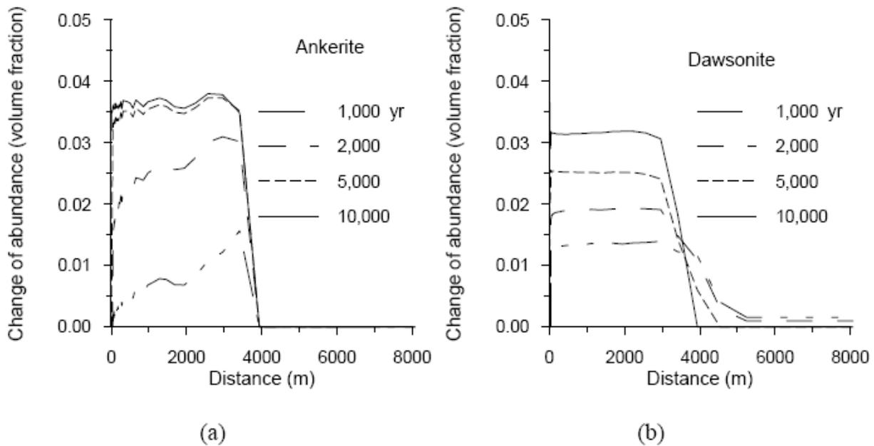
**Figure 6-17. Change in Mineral Abundance (Negative Values Indicate Dissolution and Positive Precipitation) after Different Times for the One-Dimensional Radial Flow Problem. Figure from Xu, et al., 2005. Results for the Validation and Supplied Output are Shown as One Set of Identical Data.**
