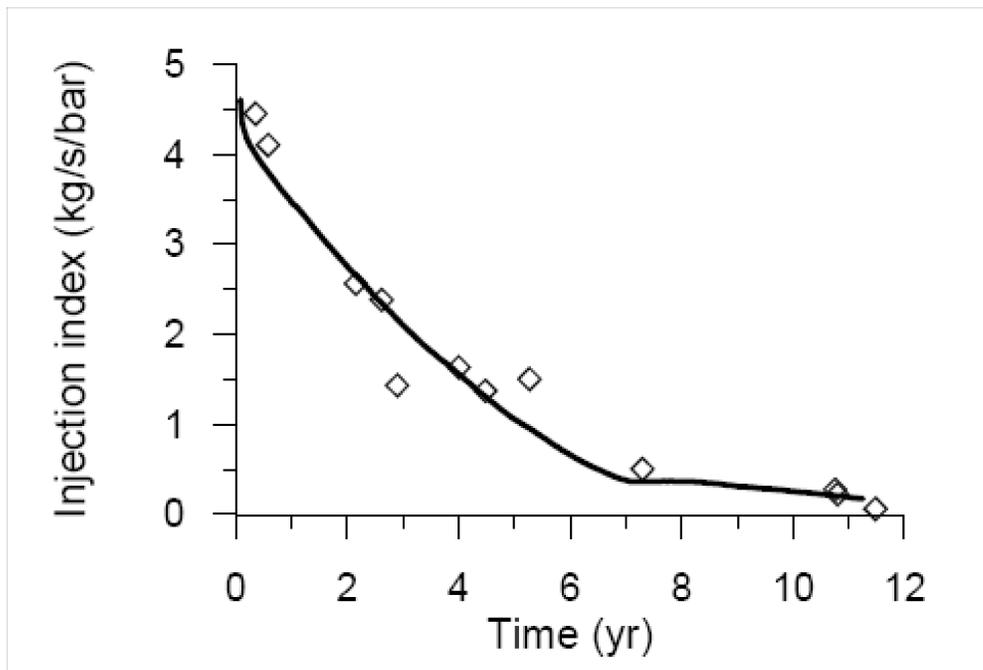
**Figure 6-31. Simulated Injection Indexes Using an Injection Temperature of 161 °C [322 °F] for the Later Time Period, Together with Measured Data (Silica Concentration = 705 ppm,  $\phi_c = 0.92\%$ , and  $n = 10$ ). Figure from Xu, et al., 2005. Results for the Validation and Supplied Output Are Shown as One Set of Identical Data.**
