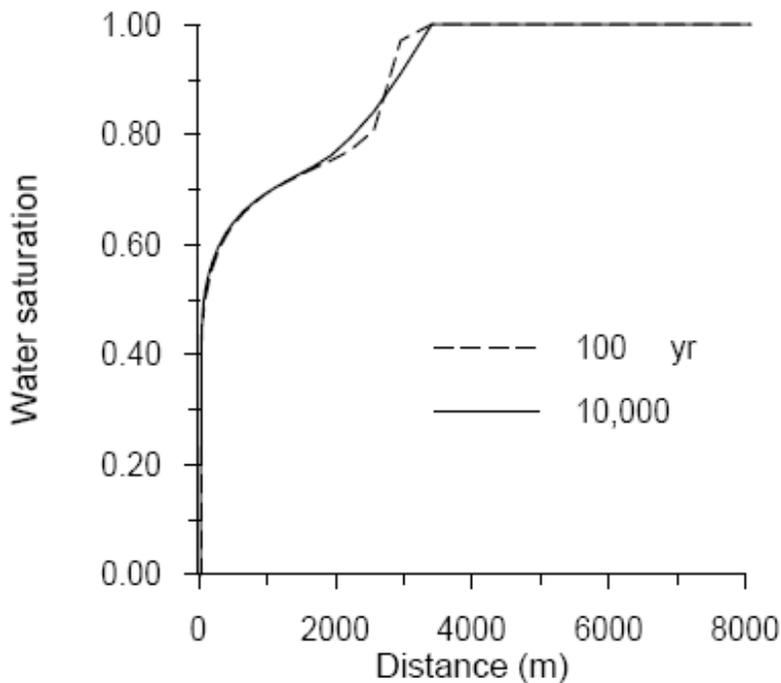
**Figure 6-16. Water Saturations at Different Times for the One-Dimensional Radial Flow Problem. Figure from Xu, et al., 2005. Results for the Validation and Supplied Output are Shown as One Set of Identical Data.**
