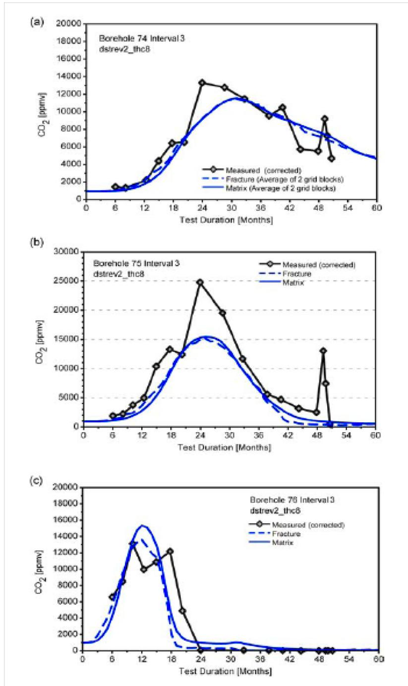
**Figure 6-12. Modeled CO<sub>2</sub> Concentrations in Fractures and Matrix Compared to Measured Values From Boreholes (Corrected for Vapor Condensation) (a) Borehole interval 74-3 (Average of Bounding Grid Blocks); (b) Borehole Interval 75-3; (c) Borehole Interval 76-3. Figure from Xu, et al., 2005. Results for the Validation and Supplied Output are Shown as One Set of Identical Data.**
