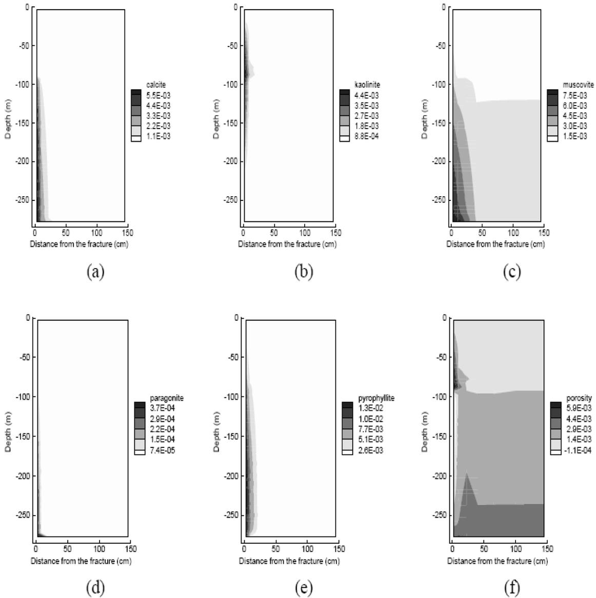
**Figure 6-27. Change of Mineral Abundance (Secondary Phases, in Volume Fraction) and Porosity after 1,000 Years. Figure from Xu, et al., 2005. Results for the Validation and Supplied Output Are Shown as One Set of Identical Data.**
