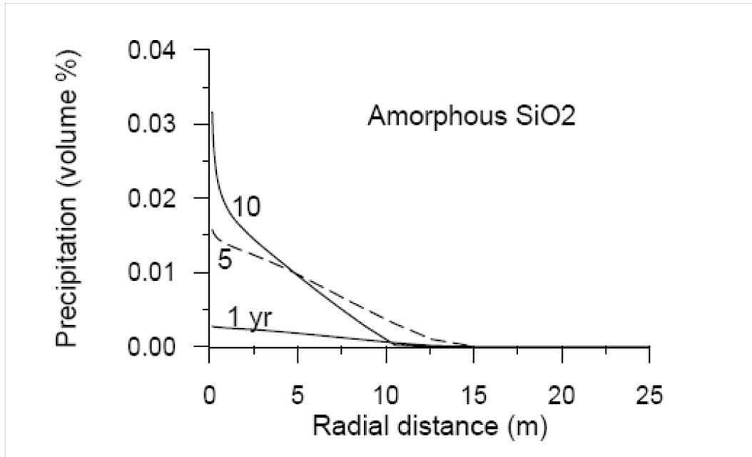
**Figure 6-33. Amorphous Silica Precipitated Along the Well Radius for the Simulation Shown in Figure 6.3.8.4. Figure from Xu, et Al., 2005. Results for the Validation and Supplied Output Are Shown as One Set of Identical Data.**
