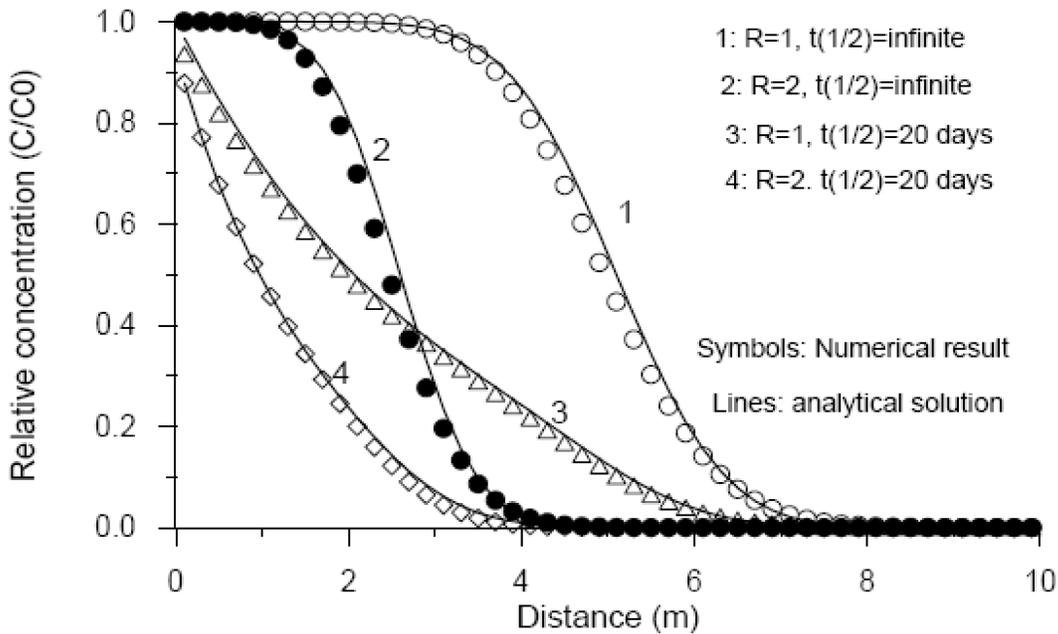
**Figure 6-2. Relative Concentrations at 50 Days for 1-D Aqueous Solute Transport with Adsorption (Linear  $K_d$ ) and Decay (Concentrations are Normalized to the Inlet Concentration of  $10^{-4} \text{ mol/l}$ ). Figure from Xu, et al., 2005. Results for the Validation and Supplied Output are Shown as One Set of Identical Data.**
