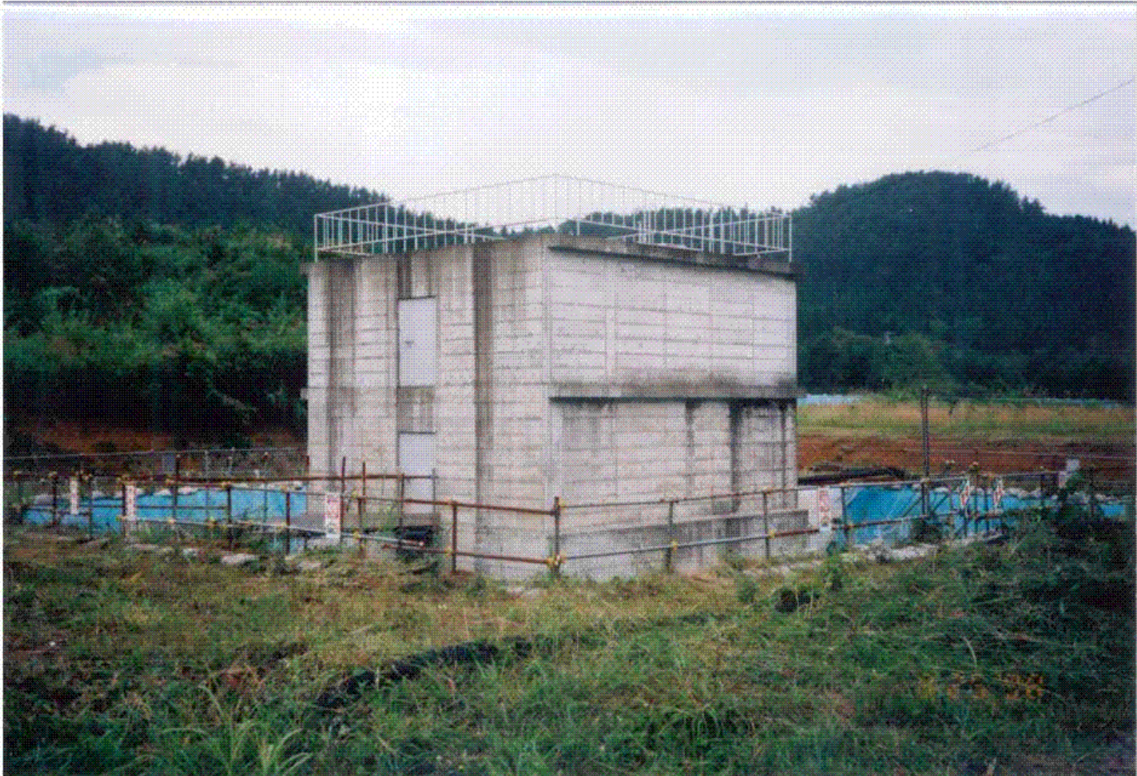
Figure 2-6 NUPEC Field Test Model of Reactor Building without Embedment
