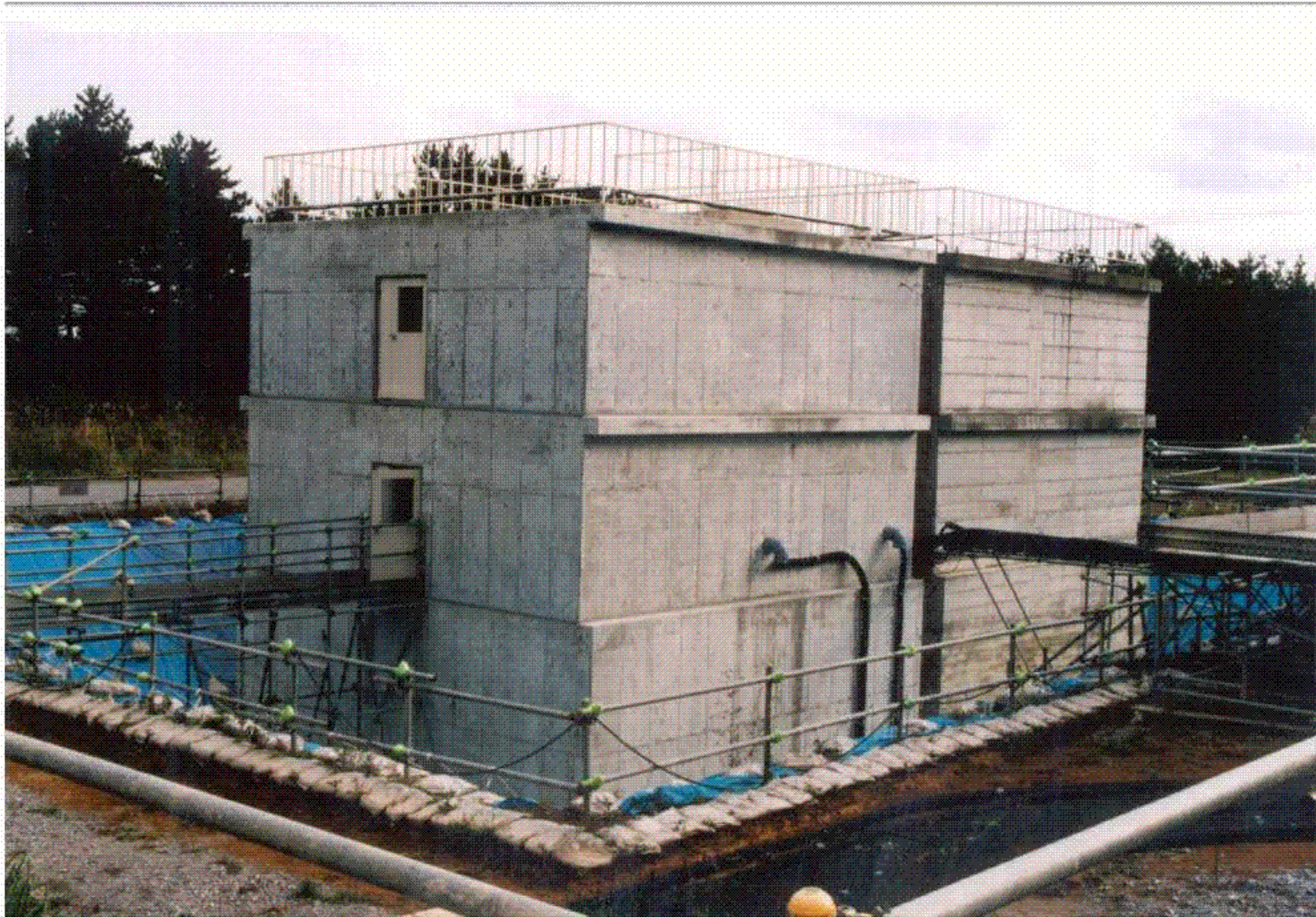
Figure 2-7 NUPEC Field Test Model of Adjacent Twin Reactor Buildings without Embedment
